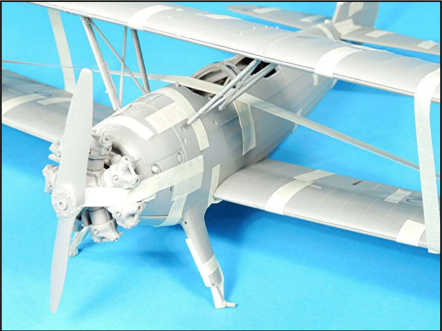
The upper wings was slightly skewed to the left because of the outer strut issues.
