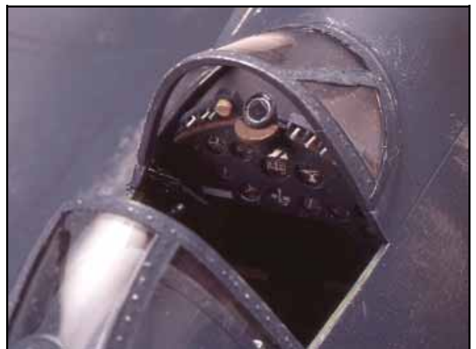
The adjustment dial to the left of the gun sight was made from a disk punched out with my Waldron punch tool. Note how the reflective lens adds realism to the gun sight.
