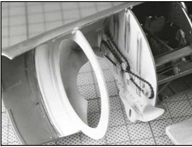
The chain drive for the landing gear was an HO scale chain from a model railroad detail set.
