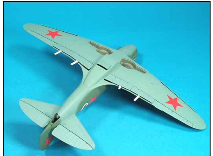
Next I installed the flaps. There are no positioning tabs for the flaps so I used pieces of plastic to position them.
