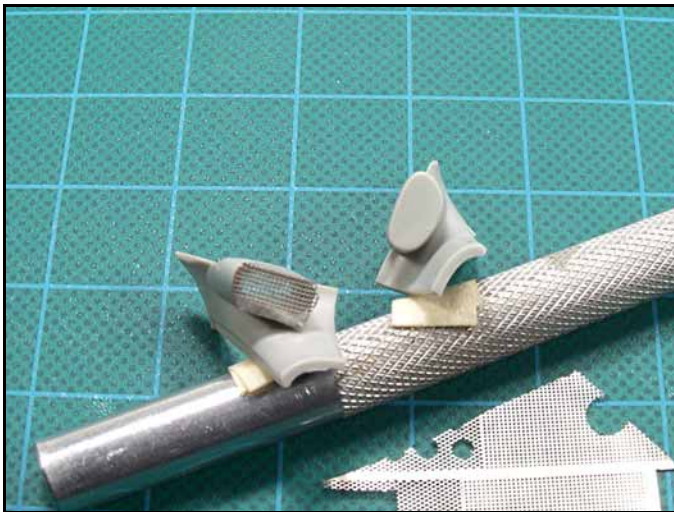
I removed the molded on air intake screening and replaced them with photoetch screening.
