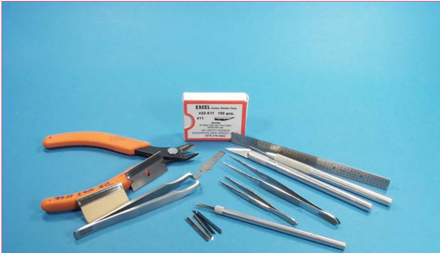
Here are the basic hand tools for snipping, cutting, trimming and scraping. The small diameter X-Acto handle and associated blades is a stencil knife. I always keep a good supply number 11 X-Acto blades on hand as well as a box of single edge razor blades and other specialty blades. The stainless steel ruler, can be found in sewing supply stores. The Tweezers and the needle tool all have a thousand and one uses in scale modeling.
