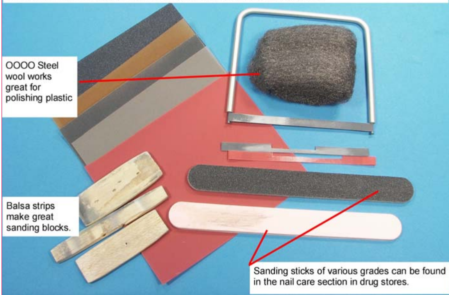
Testors and K&S Engineering sell color coded sandpaper of various grades. You can also use automotive grade sandpaper. The "U" shaped tool and associated long, narrow sandpaper strips is a Flex-I-File, which works great around contoured surfaces and round shapes.
