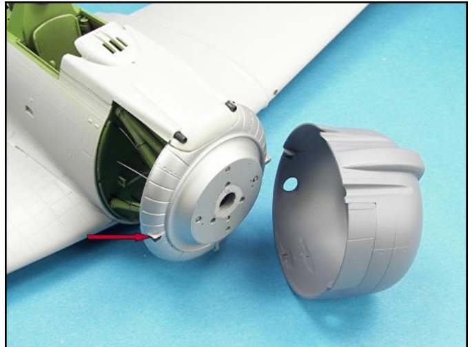
The positioning taps on the heat shield for the cowling needed to be scraped down a little so that the cowling would fit correctly.
