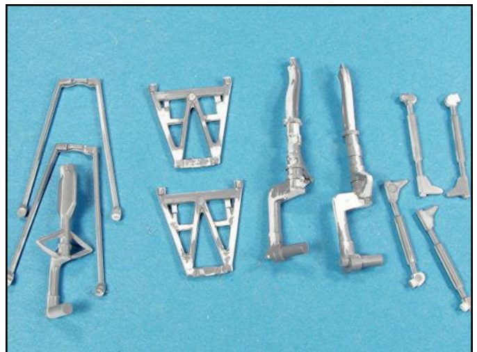
These 1/48 scale B-26 landing gear parts were white plastic. They were primed to make the mold lines and mold punch outs easier to see.
