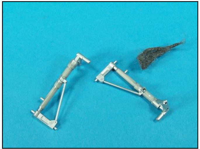
Silver paint was applied to check for flaws and then the surfaces were polished with 0000 steel wool.
