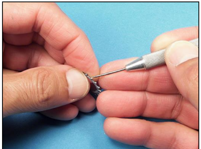
The first step in drilling out the engines wiring harness for the spark plug wires is to indent the surface for a drill bit.
