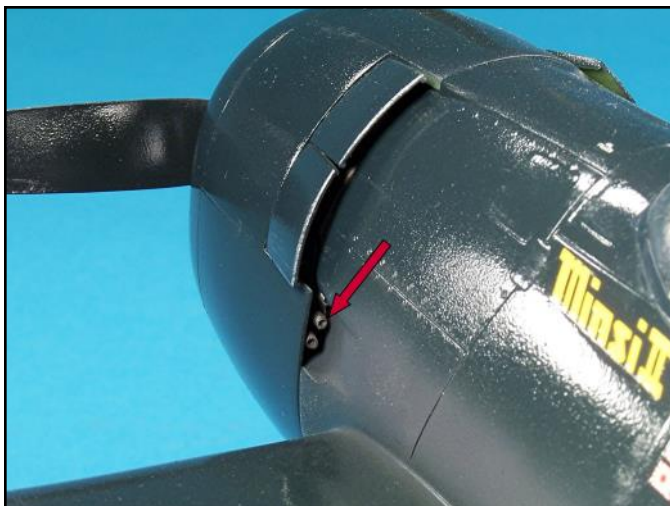
The engine exhausts on this F6F Hellcat were hollowed out using the same drilling technique.
