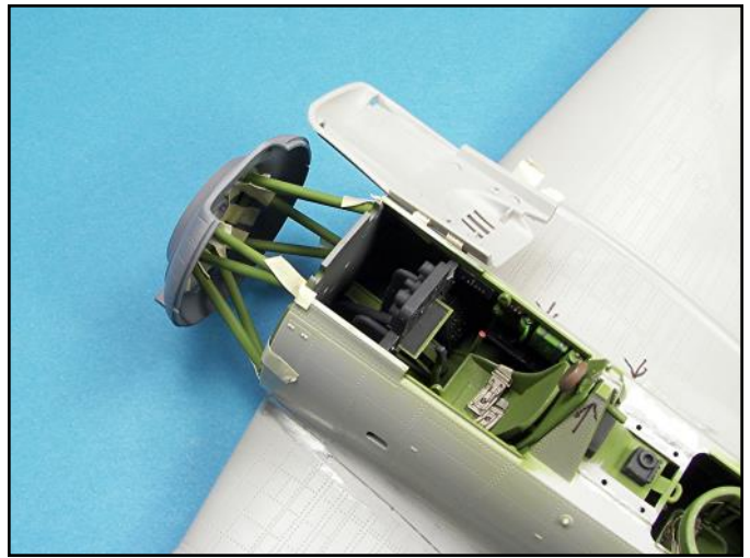
The heat shield and engine frame got a final fit check. Checking and rechecking part assemblies is the best way to prevent a misalignment problem.
