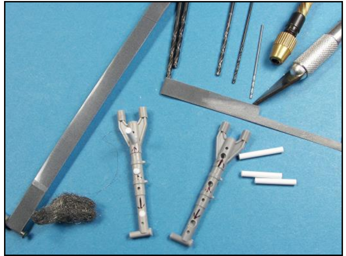
The mold punch outs on this F6F were deep so they were drilled out and plastic rod super glued into place to fill the holes and add strength to the parts.
