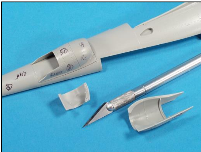
The side boom engine air intakes on this P-38 kit were multi-piece assemblies that had some fit and void challenges.
