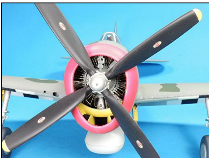
The spark plug wiring was added using brass beading wire. Note how all the colors complement one another.
