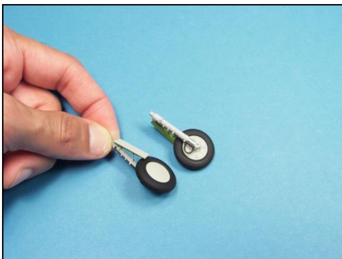
Careful masking, detail painting and airbrushing make all the difference with the appearance of landing gear, hubs and tires.
