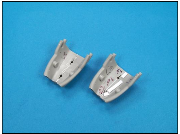
The center sections of the lower air intakes had voids that were filled with various thicknesses of plastic strips.
