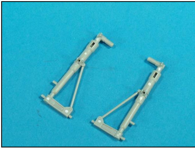
These P-38 landing gear parts had mold punch outs that were deep. I drilled the holes slightly deeper, glued plastic rod into the holes, cut the rods and carefully sanded the surface smooth, with a Flex-I-File and a sanding stick.
