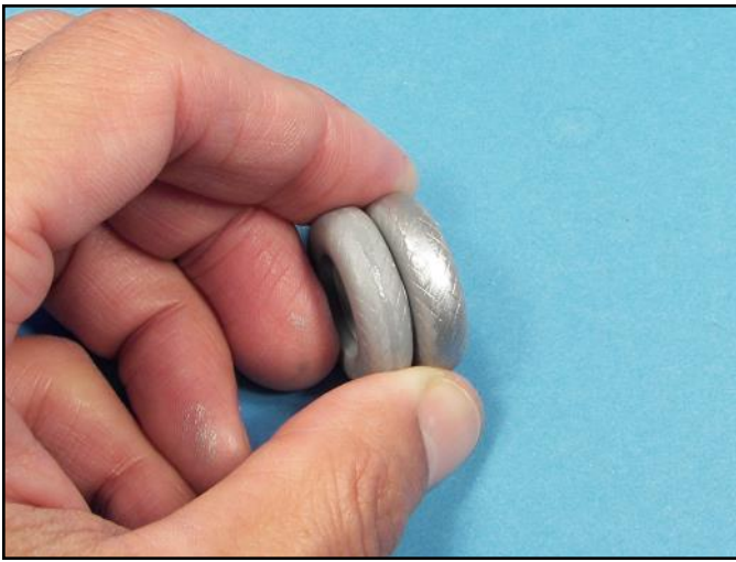
The surfaces were checked for flaws with silver paint as a last step before restoring the tread.
