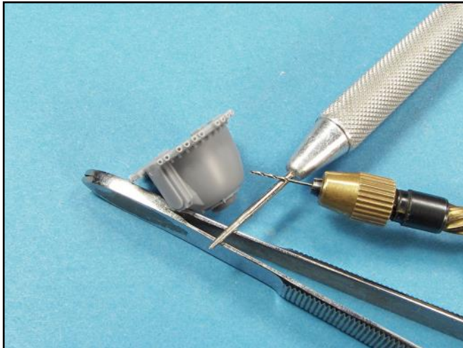
Holes for the spark plug wires were carefully drilled out using a .0145 inch (#79) drill bit. The punch was used to create an indentation in the surface of the plastic for the drill bit.
