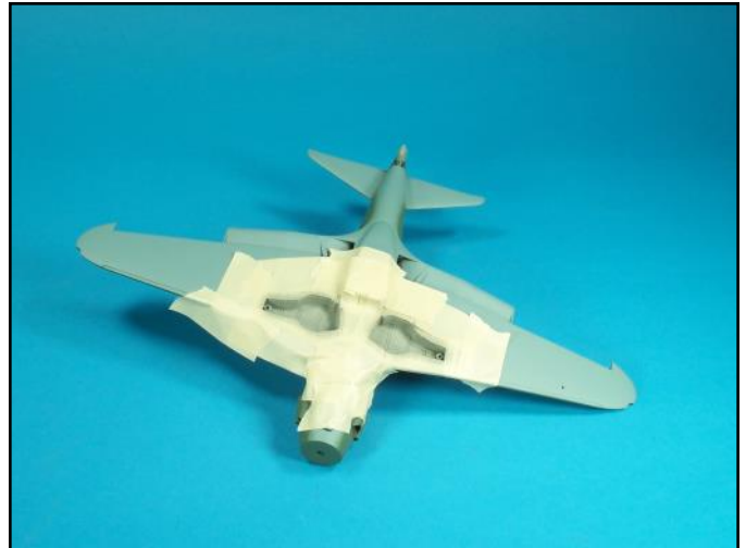
To paint the wheel wells on this Mig-3, the area around the openings were carefully masked and then larger sheets of masking tape were applied to protect the surface from overspray.
