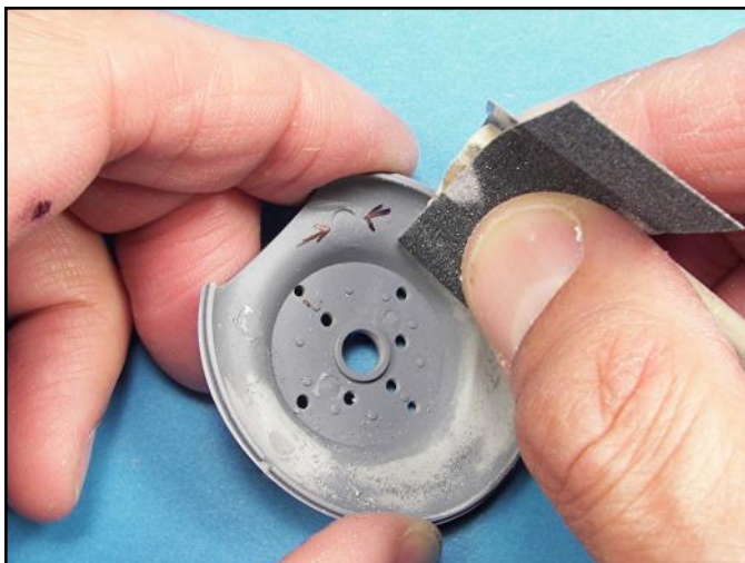
This heat shield had mold punch outs that needed to be removed. Sandpaper was wrapped around a thin section of balsa wood to get into this tight area.
