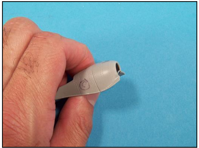
The leading edge area looks great thanks to careful applications of super glue, careful scraping and wet sanding.
