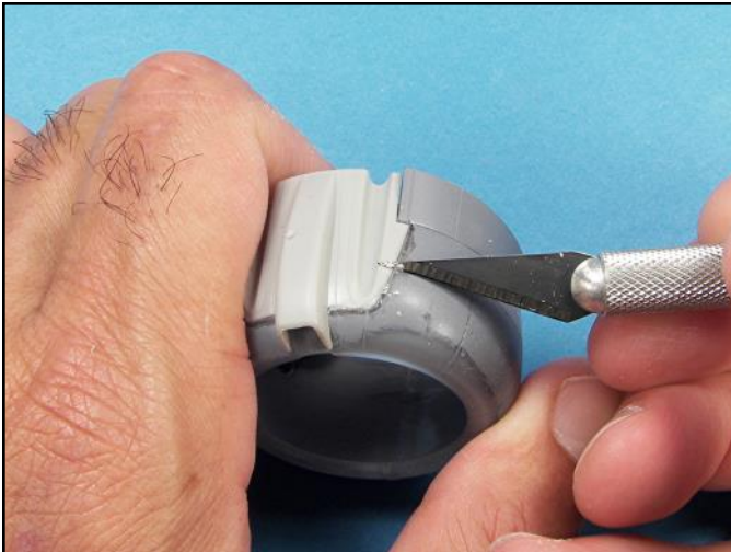
The upper cowling section was super glued into place and the seam was lightly scraped with the tip of a number 11 X-Acto blade. The plastic was then wet sanded smooth and polished with a 0000 steel wool pad.
