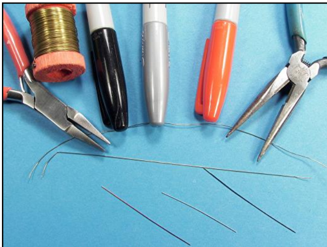
The wiring and plumbing for this engine assembly was accomplished with brass beading wire stretched straight and then painted with indelible markers.
