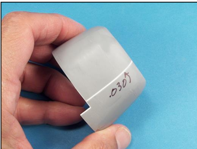
With the added strips cut and sanded smooth, the engine cowling now has the correct depth eliminating the step between it and the fuselage.
