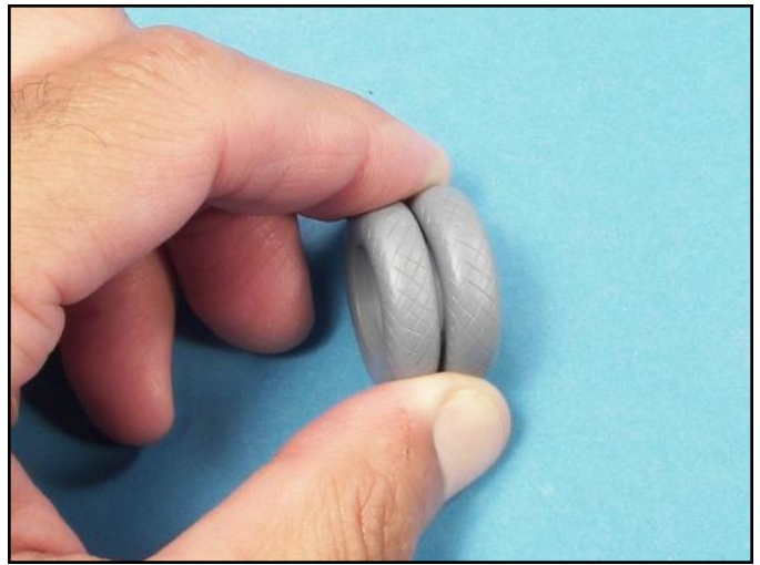
The wheels were sandwiched between two lengths of balsa wood and then placed in a Dremel vice. The tread was cut across the plastic using a jeweler's saw. Only one pass with the blade was necessary to restore the tread.
