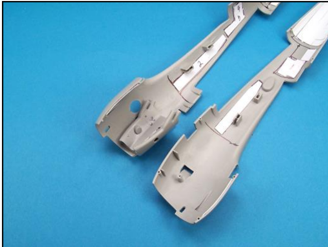
The plastic thickness on many new kits is very thin. Reinforcing the plastic by laminating sheets of plastic to the inside areas with super glue will prevent flexing of the plastic, which can crack a seam.
