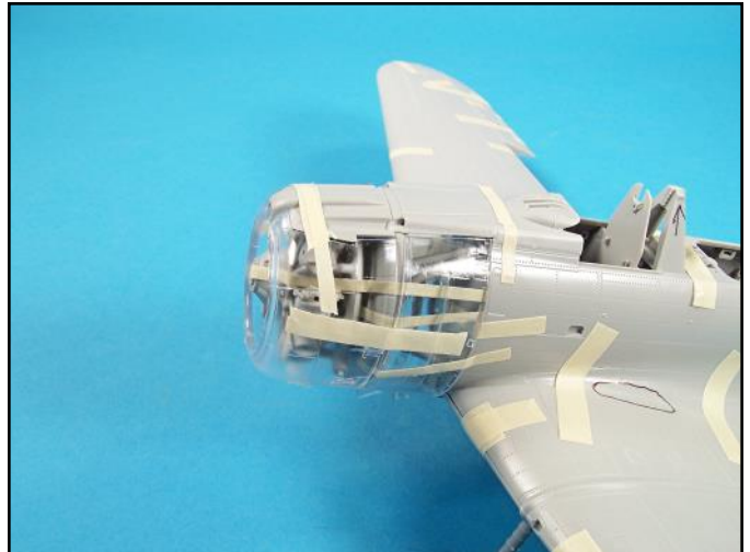
The last step in test fitting the engine is to be sure that it does not interfere with the engine cowling parts. On some kits the engine cylinder straps on the ends of the cylinders need to be thinned so that they do not interfere with the cowling.
