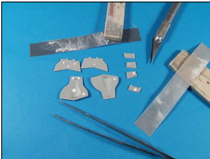
There were a lot of mold punch outs on the inside of these landing gear covers. Since the Eduard photoetch set had framing detail for these parts, the deep punch outs were filled with disks and the entire surface was sanded flat.
