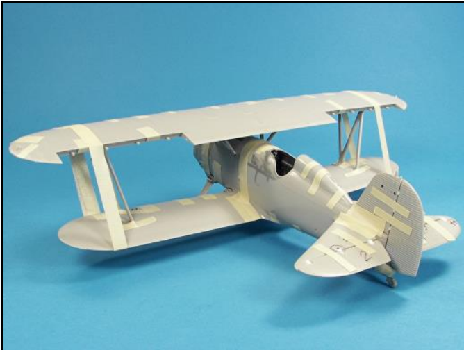
Test fitting biplanes also allows you to mark the flying wire locations and drill the holes at the correct termination points and angles.
