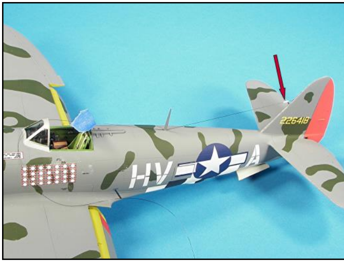
A .0145 inch hole was drilled through the base of the antenna and then the length of inked nylon sewing thread was glued into place. The insulator was made from a short length of hollowed out .025 inch rod.
