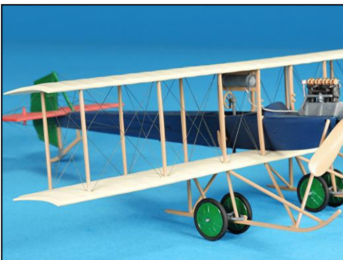
All the flying wires are tight and there are no odd crimps at their bases thanks to the angled holes that were drilled into the wings. The finished model is a great representation of a 1911 Avro biplane.
