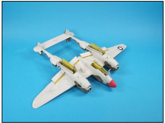
These P-38 flaps have been positioned and then glued into place. When installing multiple flaps be sure they are all set at the same angle.
