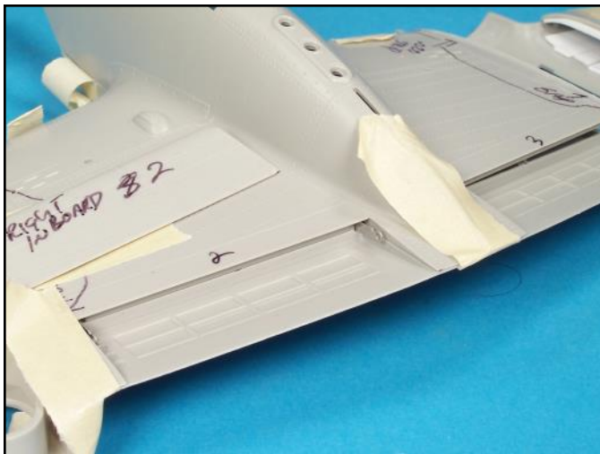
The metal tabs for the flaps were test fitted to be sure that they slid in and out.
