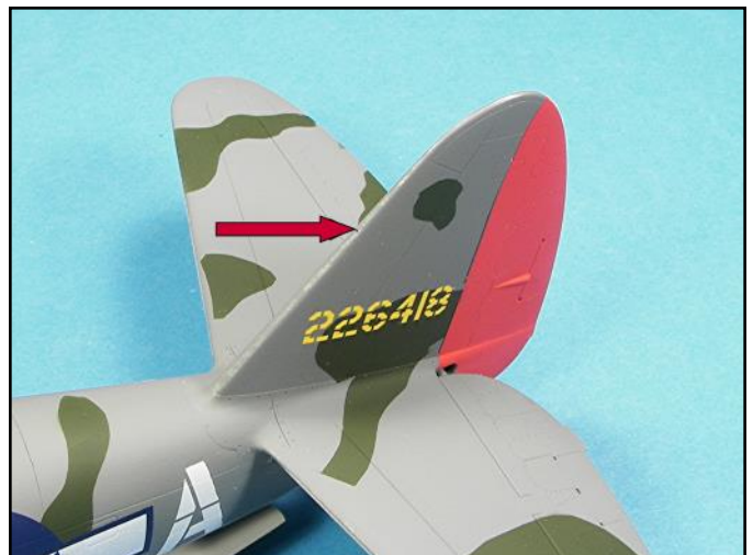
On this P-47 a .0145 inch hole (number 79) was drilled into the leading edge of the tail.
