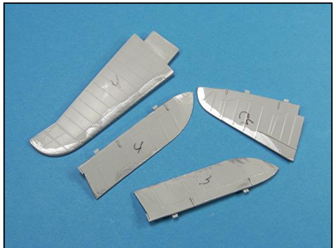
These control surfaces have been given a coat of silver paint on their seams to check for any remaining flaws. Note the parts numbering on them.
