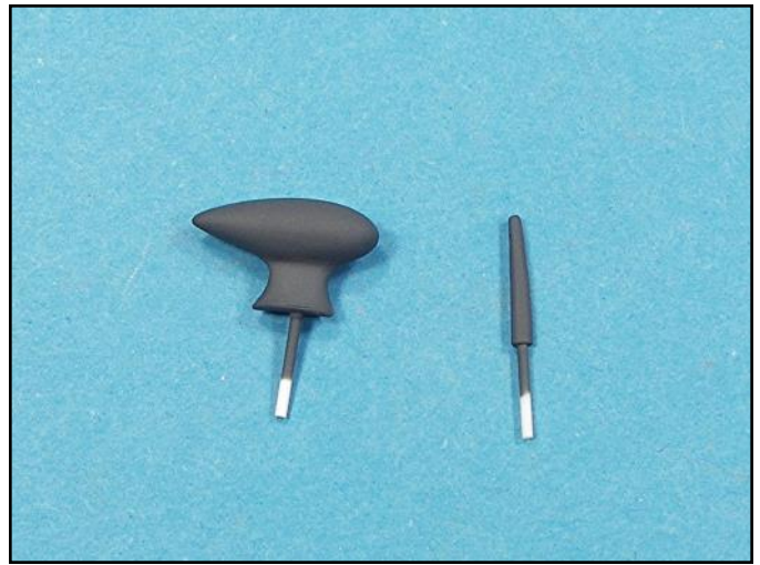
These two antennas were attached to the fuselage halves and mismatched. They were cut off and stubs attached to them for a stronger attachment to the fuselage. The post had a .0145 inch hole drilled through its tip.
