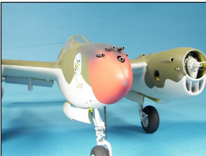
With careful drilling by hand and working up to the diameter opening you want to achieve using progressively larger bits, you can achieve very thin walls.
