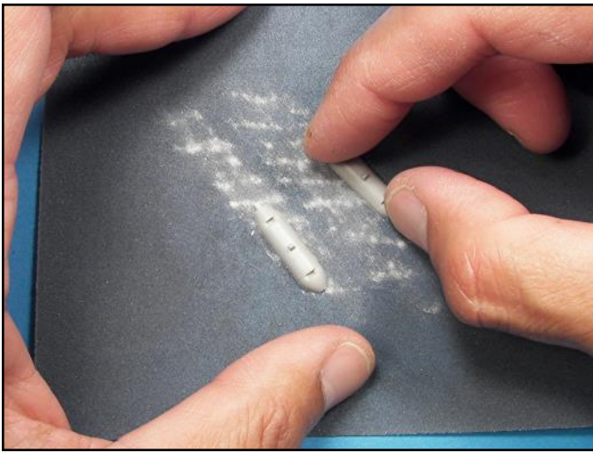
Bomb halves that are just flat can be run across a stationary piece of sandpaper to remove any irregularities on the gluing surface. Be sure to test fit the bombs together.
