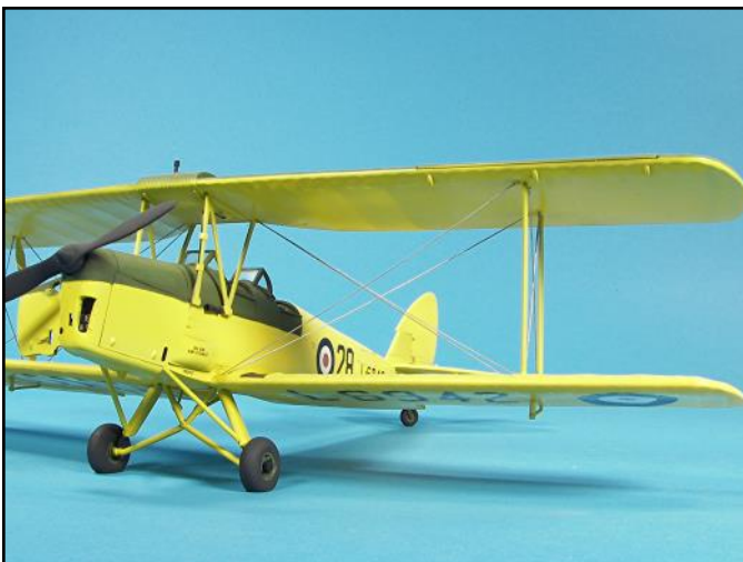
This 1/32 scale aircraft was rigged 25 years ago. The wire has not sagged, but there are tiny surface rust spots on the wire because I did not paint it.
