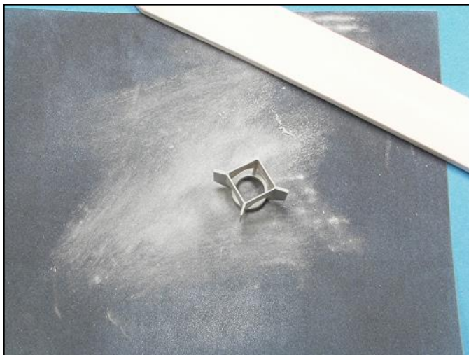
The base of the fins need to also be flattened so that they will fit correctly on the bombs.
