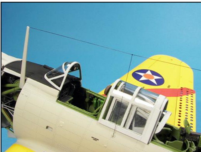
The thread was attached to the tip of the forward antenna post. A .0145 inch hole was drilled into the antenna base plate on the fuselage and a length of thread glued into place. The thread was then glued to the horizontal length.
