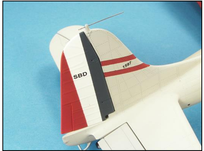
On this SBD, the antenna stub was drilled through with a .0145 inch drill bit (number 79). Inked nylon sewing thread was pushed through the hole and super glued into place.
