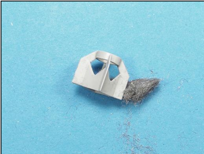
This bomb fin is assembled and the seams have been scraped smooth and the plastic polished with 0000 steel wool.
