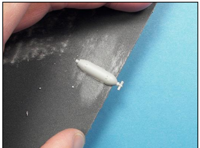
The bomb halves that have complete fuses on one half have to be sanded with the fuse area off the edge of the sandpaper.
