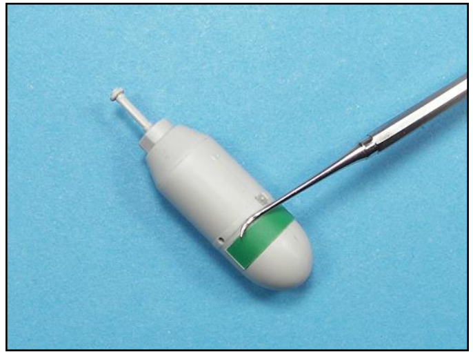
This 1000 lb. bomb has an engraved line that was marred when the seam was scraped. To restore the line use labeling tape as a guide for a panel scriber.
