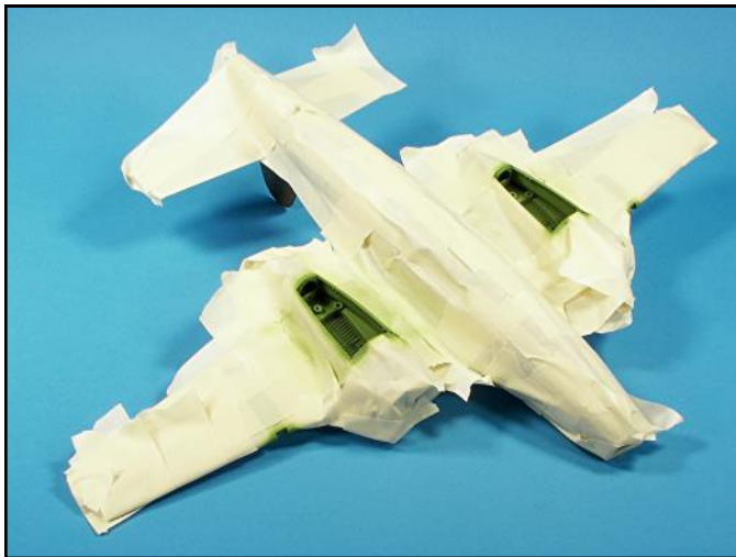
Strips of masking tape were applied around the landing gear bay openings and then the entire lower surface was masked to prevent any overspray or paint bleeding.
