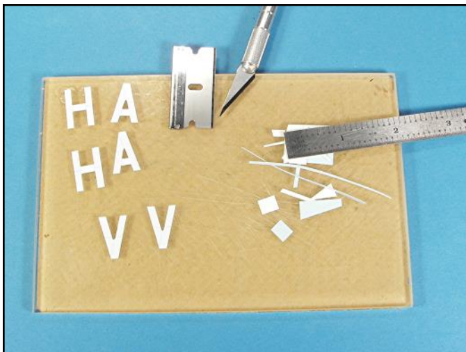
For clear film inside numbers such as "6" or letters such as "A" you will have to free hand the cuts, so go slow and check your work as the cut progresses.
