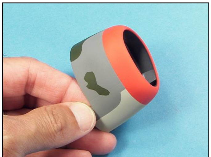
The same paint layering techniques used on the fuselage was also used on the engine cowling.
