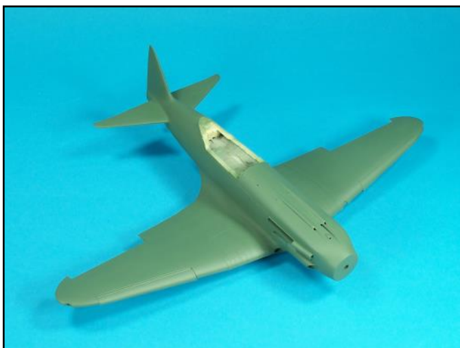
The wing and tail edges were masked and the upper surfaces airbrushed Russian green. A Badger 200 detail airbrush was used to free hand the green and blend it into the underside blue.
