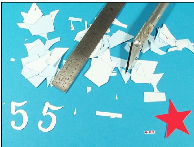
Even with the surface of a model coated with a clear gloss, there is a chance that tiny areas of a decals clear film will silver. To minimize this remove as much of the clear film as possible.
