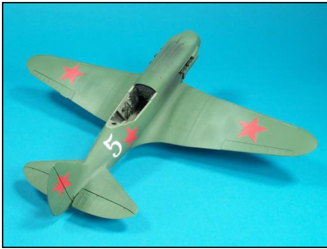
The surface of this Mig-3 was airbrushed with a highly dilute mixture of water based flat white to fade the surface paint color and the decals.
