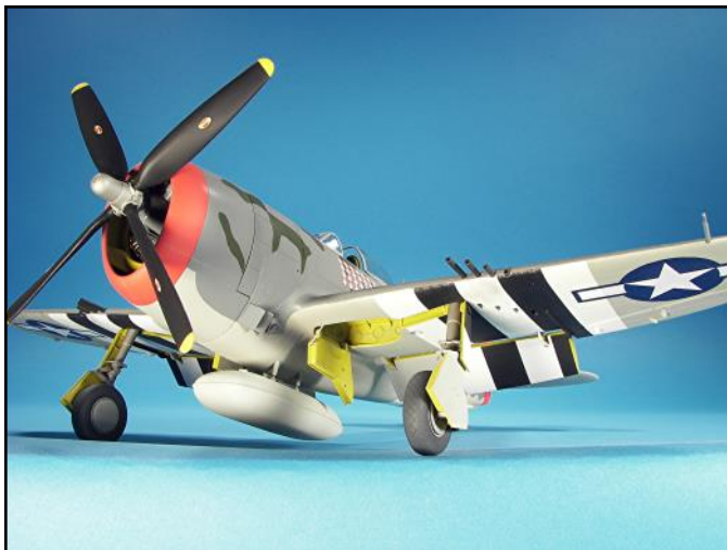
The exhaust staining on this P-47 should have been slightly darker and there should have been some discoloration around the exhaust ports due to high temperatures.
