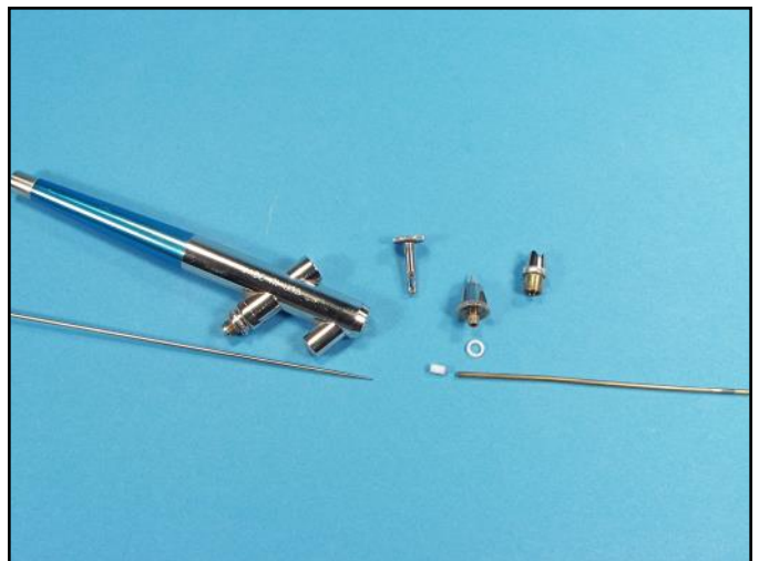
The Teflon needle bearing and the Teflon washer on my Badger 200 single action airbrush get replaced every six months.
