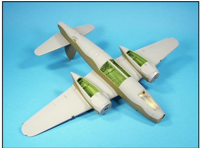
Here again, all the masking tape was removed to check for any paint bleeding or over spray of the interior color onto the outer surface.
