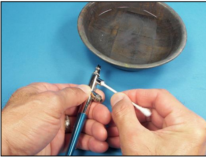
To clean the bottom feed of a Badger 200 airbrush use Q-tips soaked in thinner.
