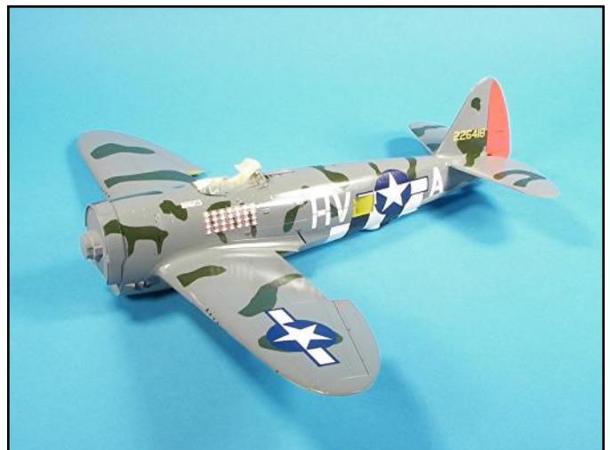
The large letters on the side of the fuselage were cut out and all the clear film removed. Having the ability to slide a decal around ensures that you have some working time to get them level and evenly spaced.
