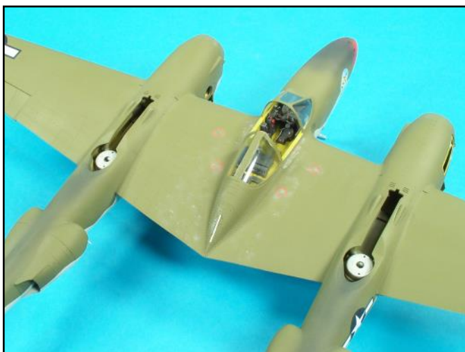
Worn surface paint due to foot traffic is very prevalent on aircraft such as the P-38 Lightning.
