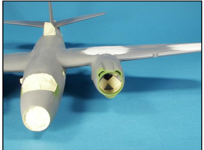
The interiors of the engine cowling were painted and then carefully masked. They were then attached to the engine nacelles with larger strips of masking tape so that the upper and lower finished color demarcation lines would match.
