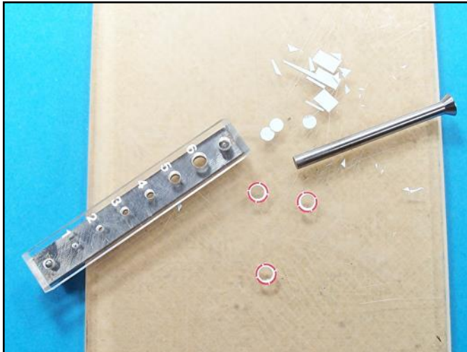
To remove the clear film from the center areas of these fuel cap decals, use a punch tool.
