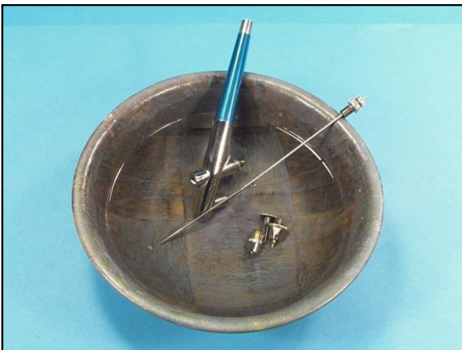
Disassemble your airbrush and soak it in thinner after each use to remove all the flakes of dried paint.
