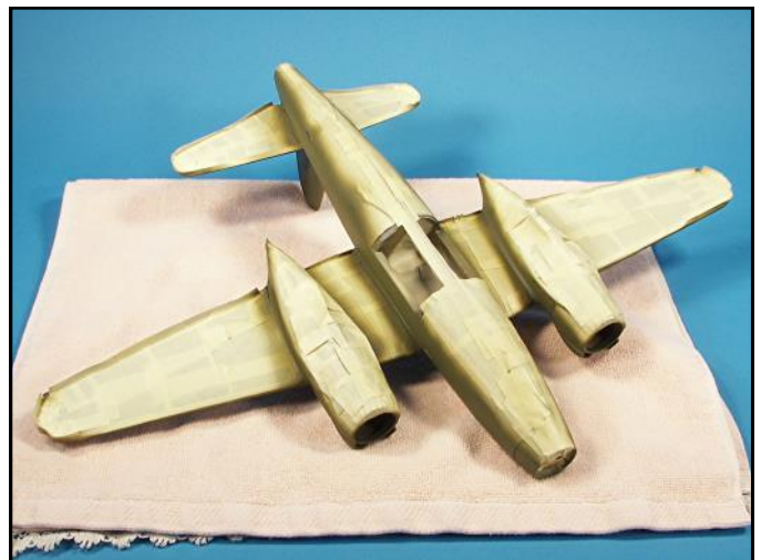
Patterns were cut on cardstock for the lower fuselage and the engine nacelles. The patterns were transferred to masking tape and applied to the surfaces. The masking was completed and the olive drab color was then airbrushed.
