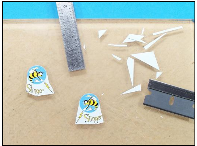
A metal straight edge, a number 11 X-Acto blade and a single edge razor blade were used to remove the clear film from around the perimeter of these fuselage nose art decals.
