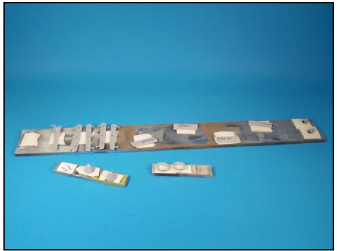
All the remaining P-38 kit parts were airbrushed using large sections of balsa wood. Sections of masking were folded over so that the tape would stick to the wood and allow the parts to also be attached for airbrushing.
