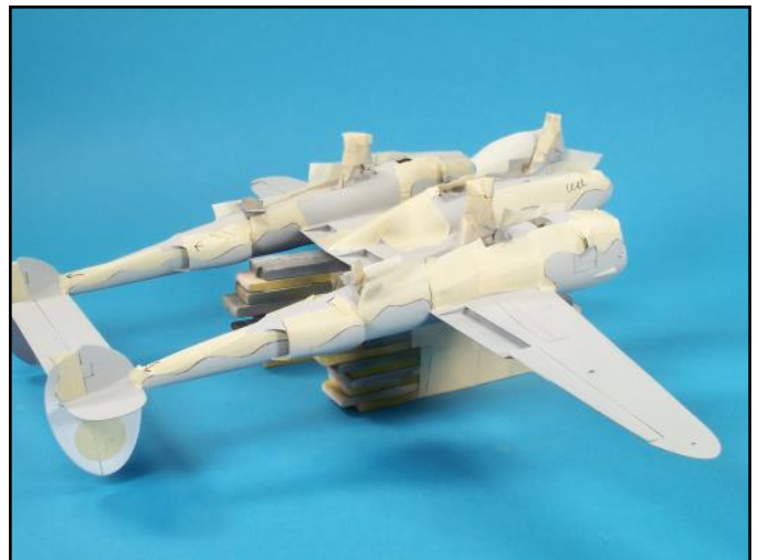
With the shaped masking tape sections applied to the fuselage and the booms, the remaining exposed areas were then masked.
