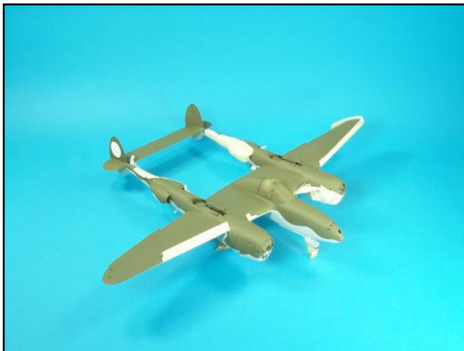
Areas were masked off where there was some olive drab paint bleeding and overspray. The pressure on the airbrushed was reduced to 10 PSI for this touchup work.
