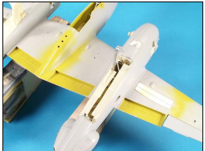
The engines and open panels were masked first. Then the landing gear bays. Masking tape was applied along the edges first.
