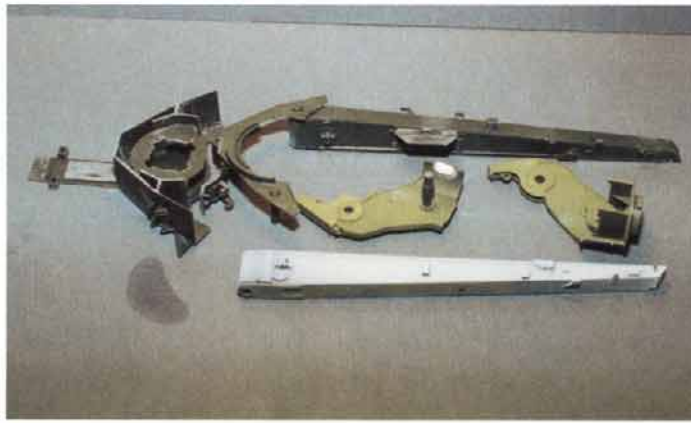
The cradle base and framing on this ARV Long Tom is starting to take shape. Model by Richard Boutin, Sr.
