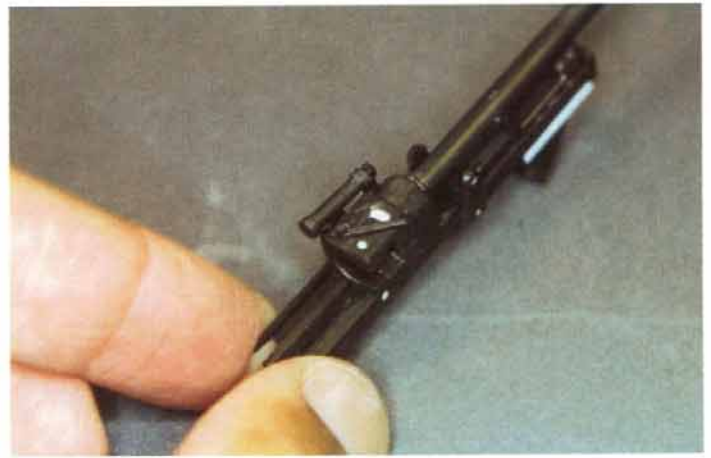
The breech assembly on this German 75mm antitank gun had injection marks and dimples that were in very tight locations. The solution was to cover them with small bits of Evergreen stock and disks punched out with a Waldron punch tool.
