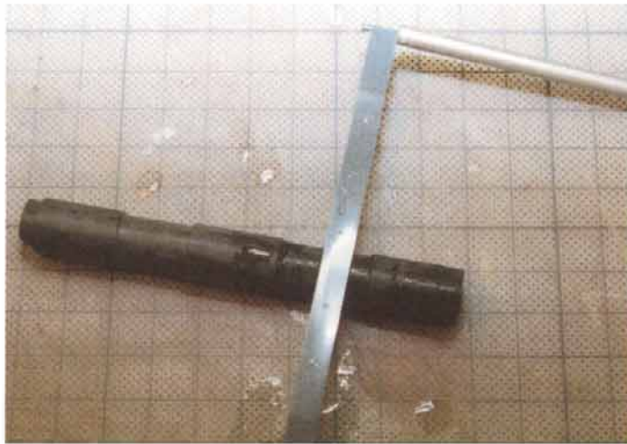
A Flex-I-File comes in handy when you need to sand around gun barrel reinforcing rings.
