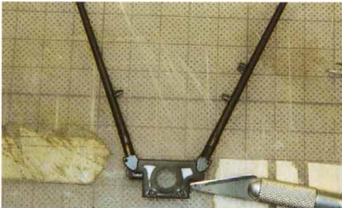
Test-fitting and assembly on small-caliber towed guns is pretty straightforward. Typically, the base and framing are single pieces that do not require a lot of assembly. The real challenge of this kit was dealing with the sink holes and injection marks.
