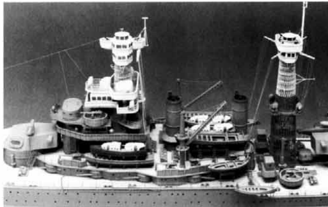
The portholes on the hull, superstructure, and small boats of Commanders Models 1/350 scale California are well done, but drilling them deeper provides for a greater perception of depth as well as perfectly rounded portholes. Model by Lonnie Ottzen, photo by Glenn Johnson, master pattern designed by John Ficklen.
