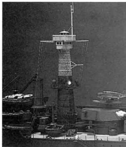
The complex and busy appearance on Commanders Models 1/350 scale USS California is achieved largely with photoetch. Model by Lonnie Ottzen, master pattern designed by John Ficklen, photo by Glenn Johnson.
