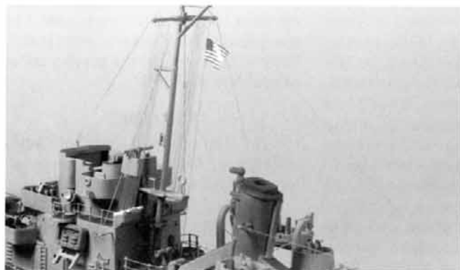
Sometimes a model needs additional details. A small length of brass wire added to the side of the superstructure provides a strong attachment point for the additional rigging that was necessary on this model.
