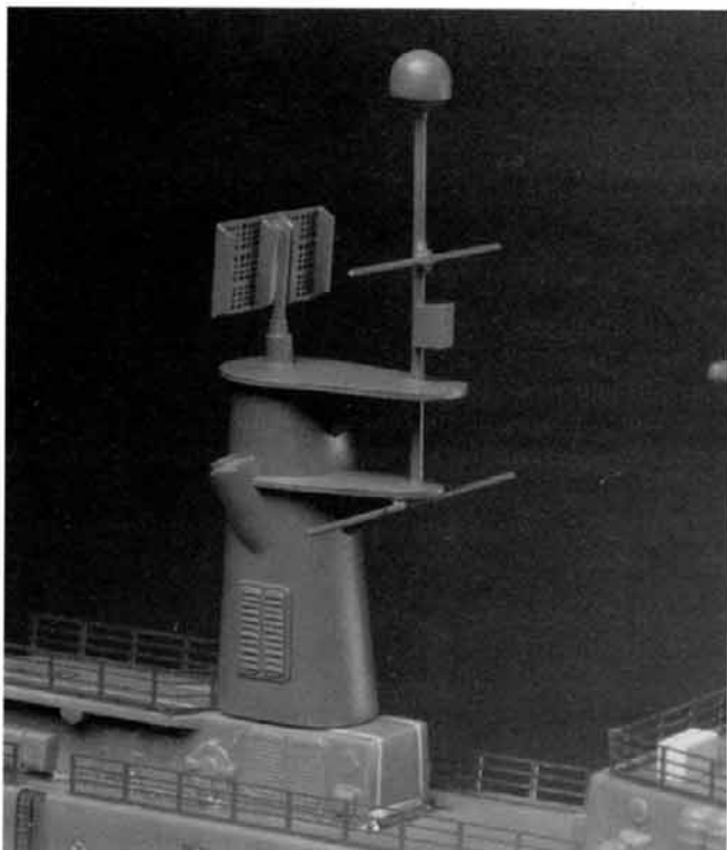
The completed scratchbuilt mast with kit parts attached has been primed and is getting its final fit check. Photo by Glenn Johnson.
