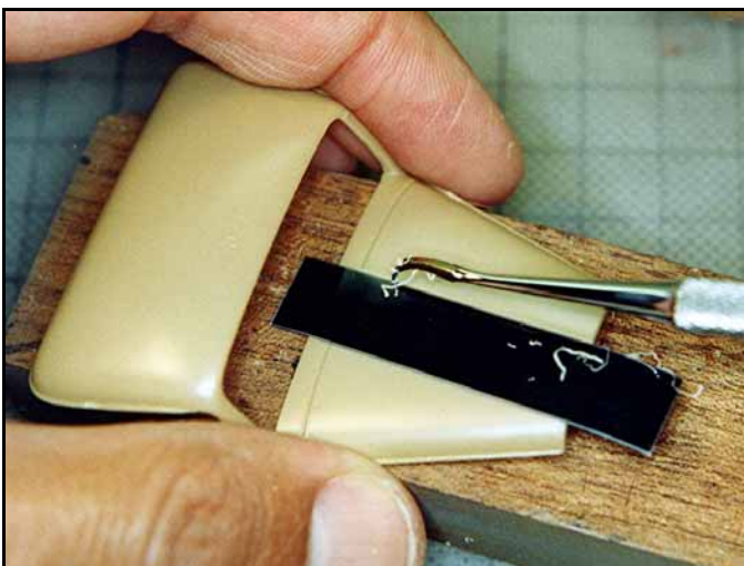
I used my trusty Bare Metal Foil plastic scribe to cut out the hood. I used labeling tape to guide the tip of the scribe.
