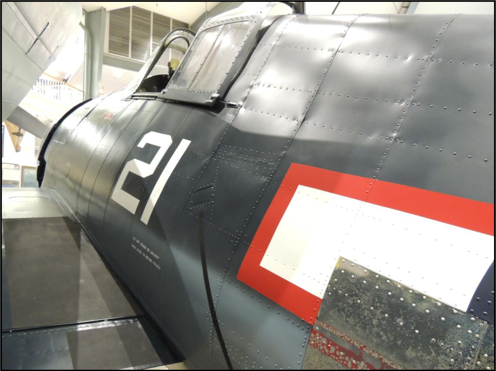
Lap joints are typically characterized by a single row of rivets.
