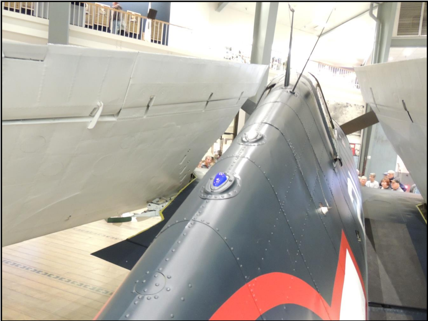
This picture shows the vertically lap joints and the horizontal lap joint along the upper spine of the framing. The surface sheeting was applied to the aft area first and then sections were applied along the fuselage over lapping one another. Note that the exposed sheeting edges face aft so as not to disrupt the airflow over the fuselage. On any scale model of a Hellcat these raised edges should be represented with raised panel lines.
