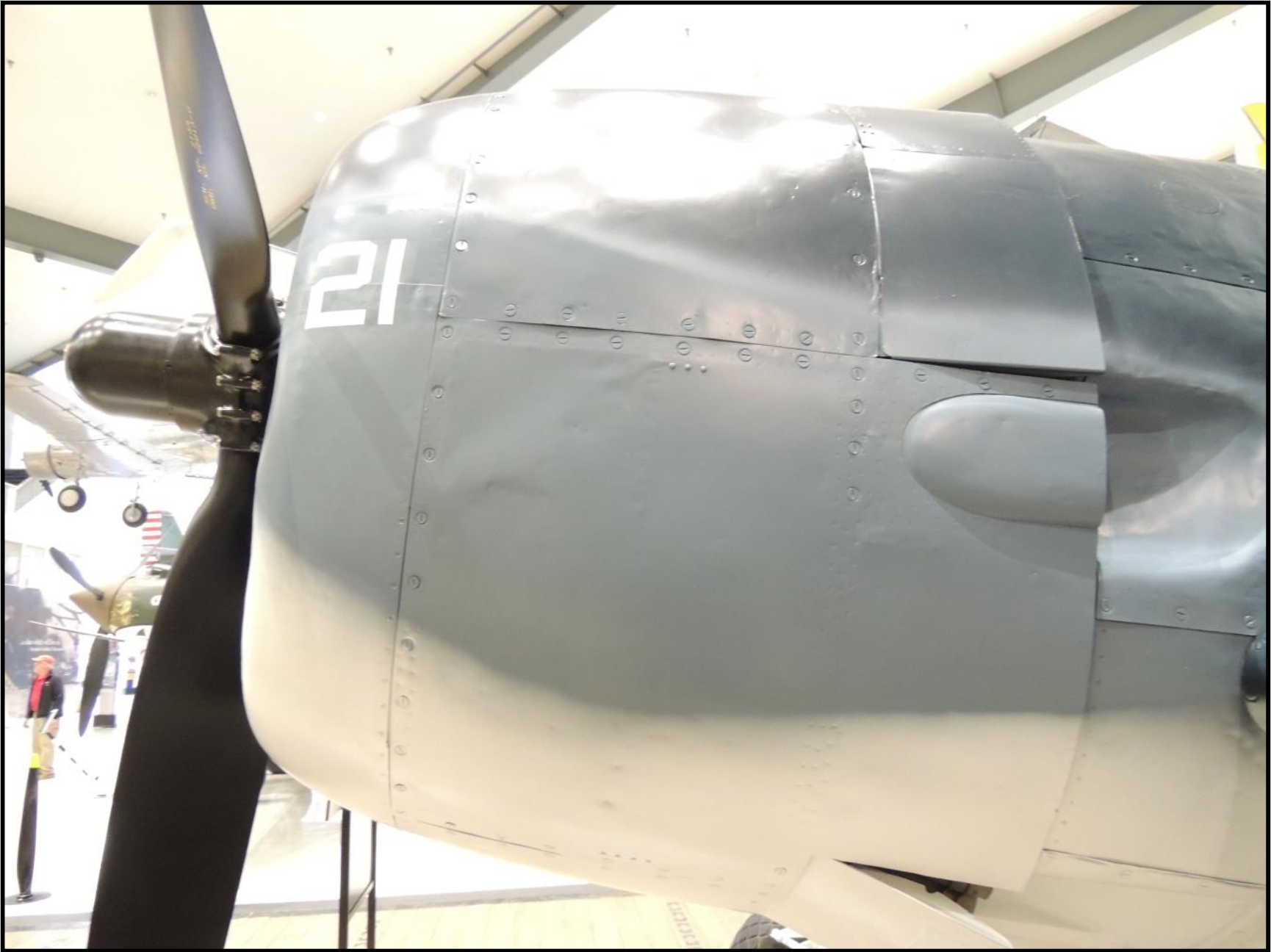
Butt joints on aircraft are represented as channels on scale model aircraft or what we commonly refer to as recessed panel lines.
