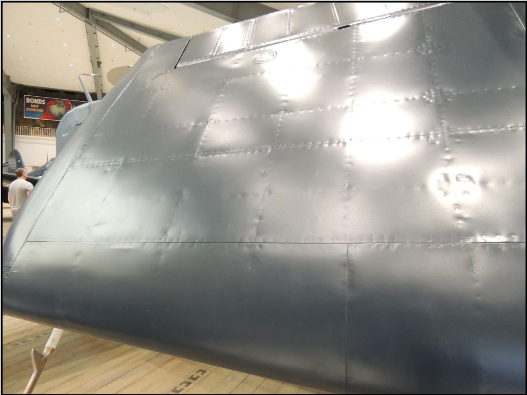
The main wing sheeting is also butt jointed with flush rivets. The channels between the butt joints are very tight and slightly less than 1/16 of an inch. Note the depressions in the surface skin due to the flush rivets. Here again the scale model recessed panel lines should be approximately .0026 inches in width and depth.
