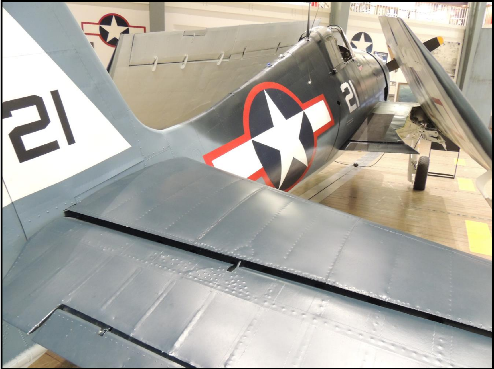
Note how the flush rivets create slight indentations on the surface skin.
