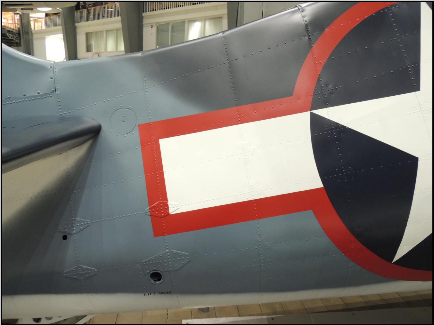
The raised shapes are reinforcing plates, which add structural strength to the aircraft's framing.
