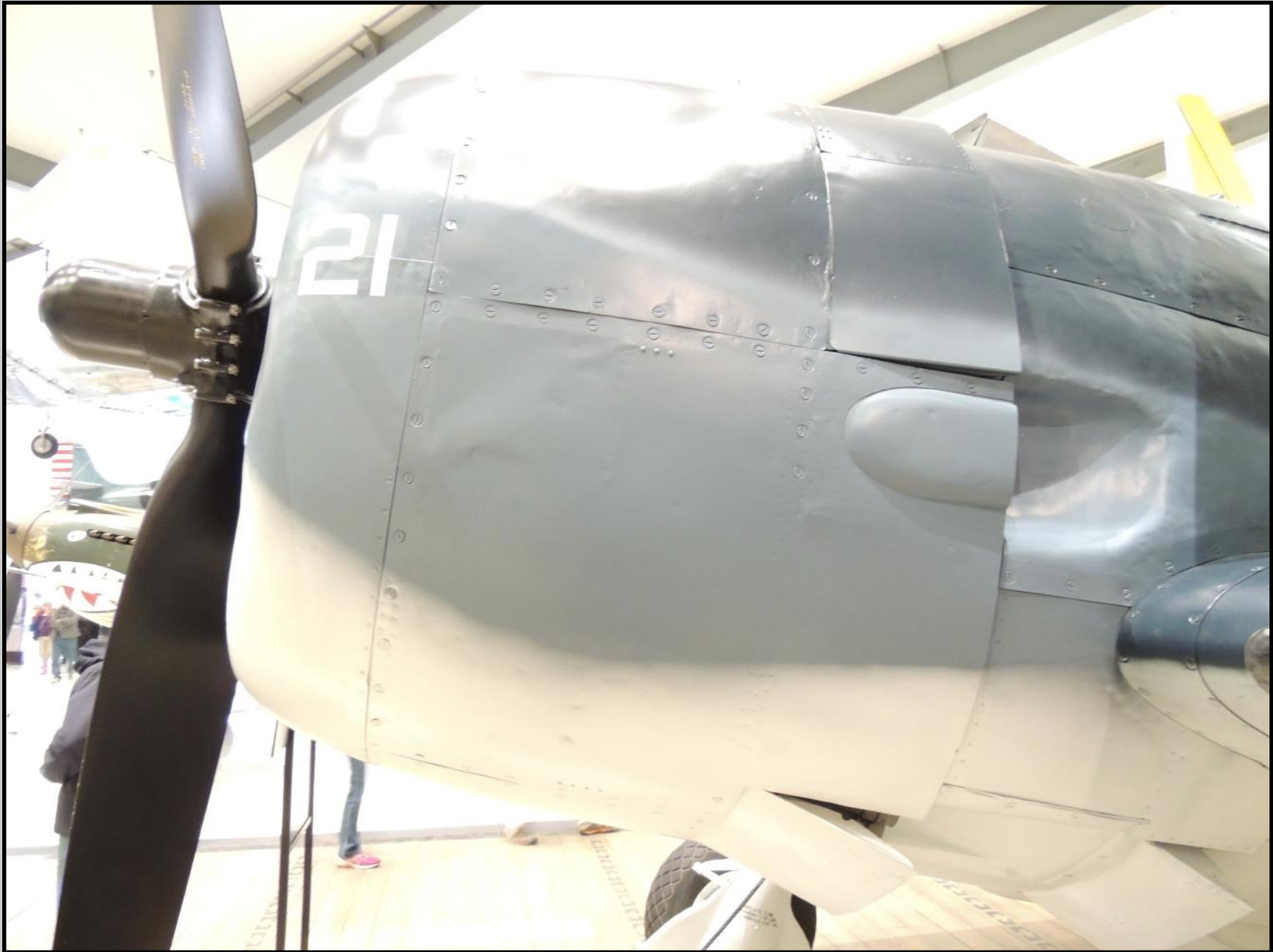
Aircraft skin is either butt jointed or lap jointed. On the F6F Hellcat the cowling engine access panels are butt jointed. The spacing between the access panels is approximately 1/16 of an inch or .0625 inches. In 1/24 scale , the 1/16 inch spacing would be approximately .0026 inches.
