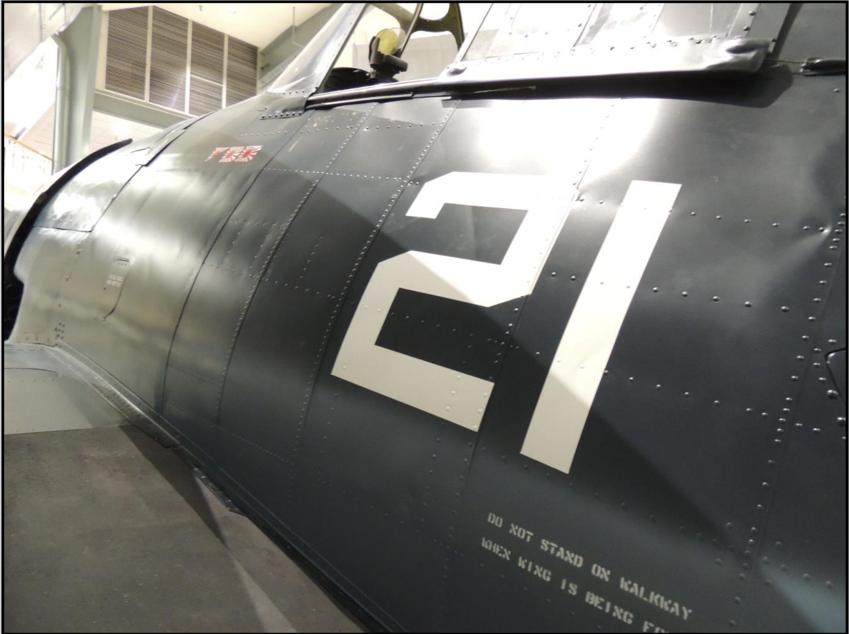
Starting at the aft end of the canopy windscreen, the fuselage of the Hellcat is all lap jointed with standard rivets. The rivet heads are approximately 1/4 of an inch or .25 inches. In 1/24 scale the rivet heads would be approximately .01 inches in diameter.
