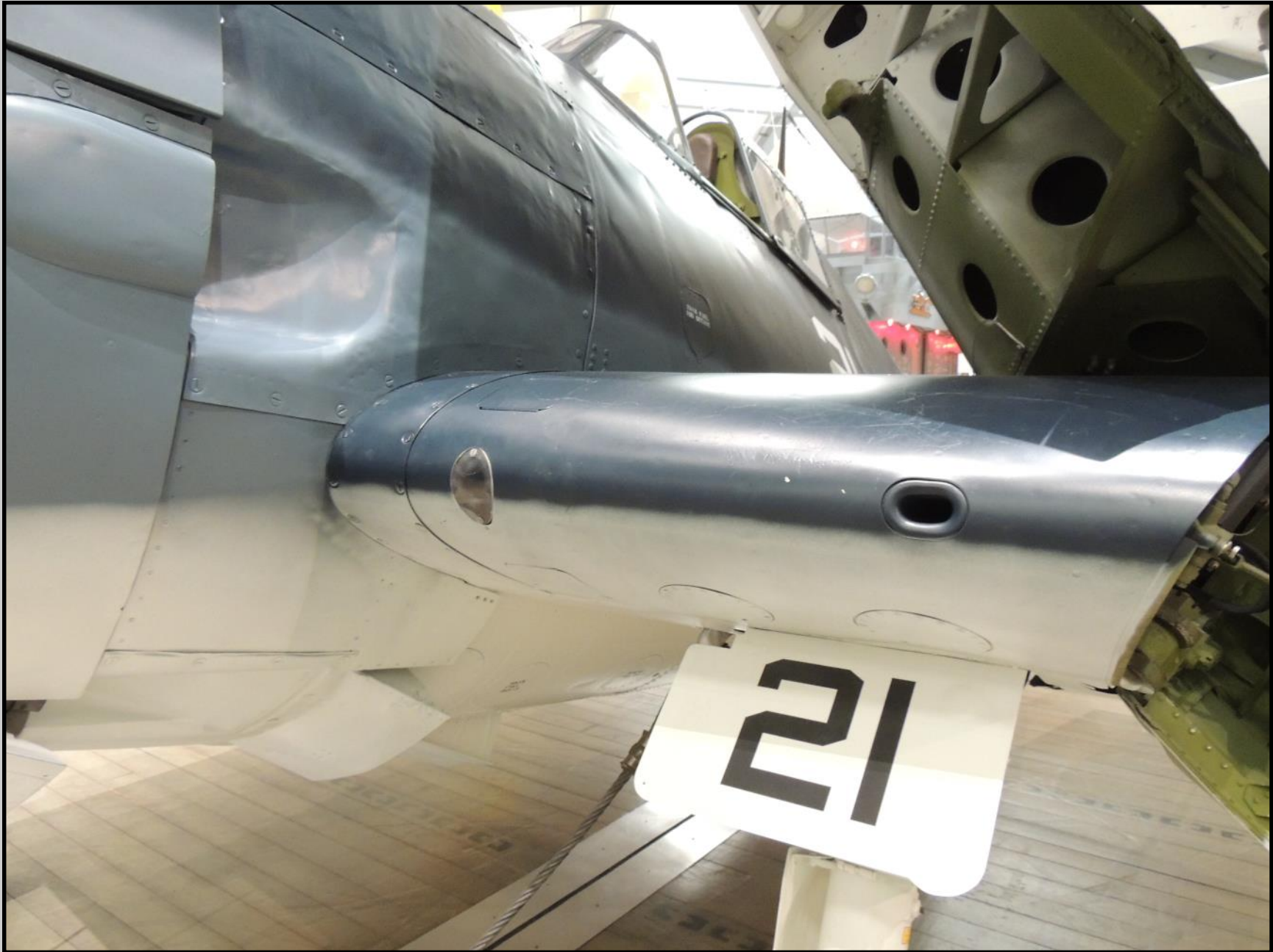
On the F6F Hellcat the aircraft's skin is both butt and lap jointed with both flush and raised rivets. On a 1/24 scale Hellcat model, the butt joints should be represented by tiny recessed panel lines approximately .0026 inches in depth and width and tiny depressions approximately .01 inches in diameter for the flush rivets. Lap joints should be represented by tiny raised panel lines approximately .0026 inches in height and width and tiny raised rivet heads approximately .01 inches in diameter.
