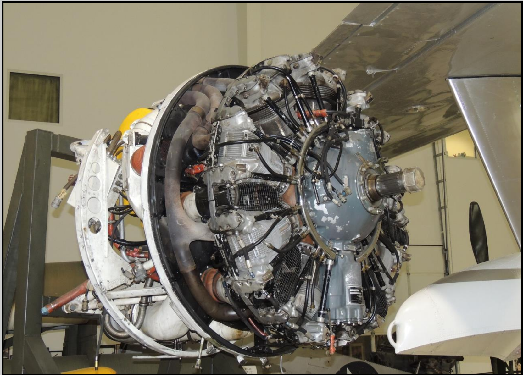
This 9 cylinder Lycoming radial engine is located at the Tennessee Museum of Aviation in Sevierville, Tennessee,
