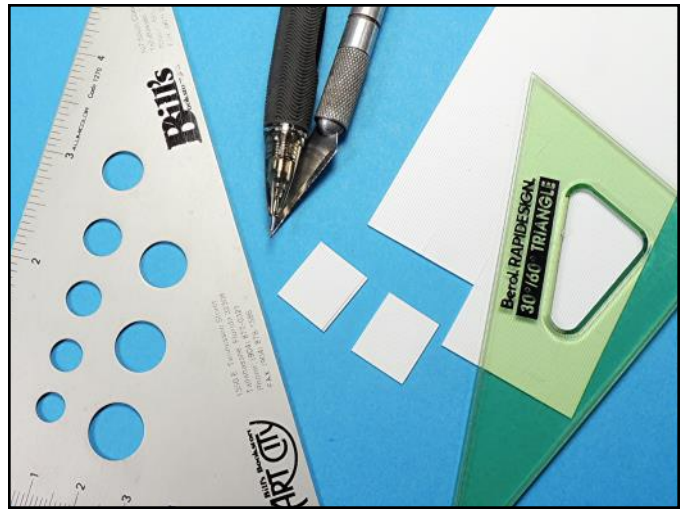
I used Evergreen .025 inch "V" groove plastic for the doors. Each door was approximately 19/32 inches long by 3/8 inches high.
