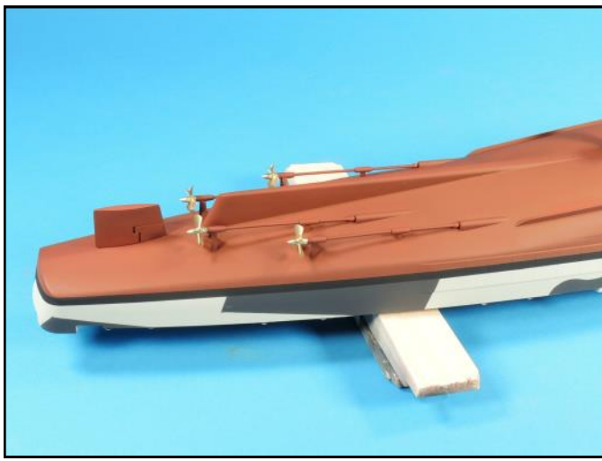
To start the final assembly process I attached the props, which were airbrushed Testors brass, with Testors tube glue.
