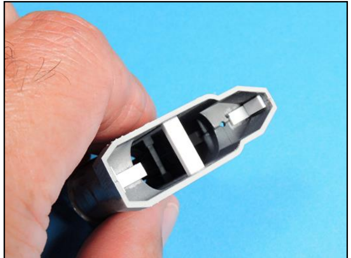
The interior of the stack was reinforced prior to working on the seams.
