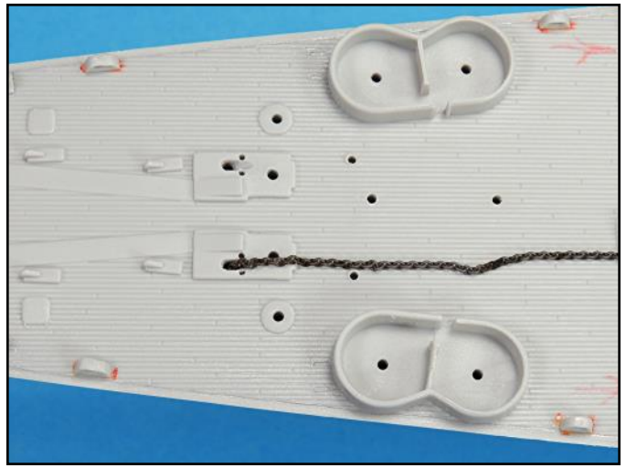
For the anchor chain to sit correctly the chain holes needed to be drilled out slightly larger and angled with a .039 inch drill bitt so that the chain would sit flat. This also helps position the chain around the capstans correctly.
