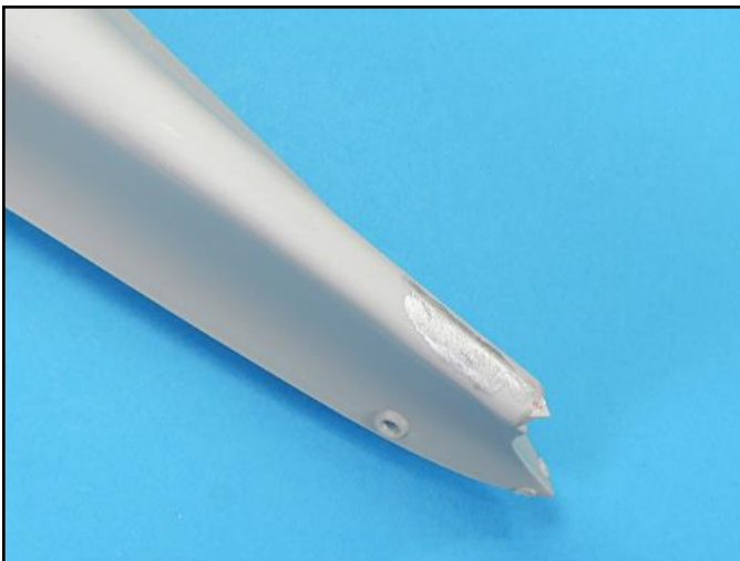
I always use Testors enamel silver paint as a flaw detector. Additional applications of super glue can be applied onto the paint and when wet sanded, the silver paint will act as an indicator when the excess super glue is sanded away.
