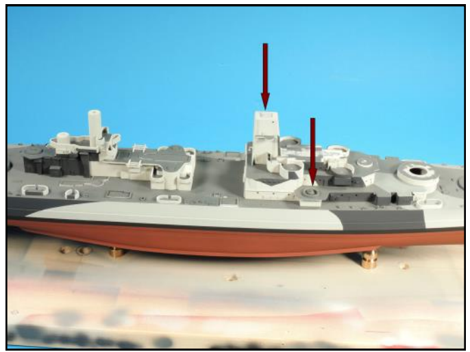
The aft superstructure was glued down first. The forward superstructure had to have some pressure applied at these points to get it to fit tightly to the deck. Note that the port side 5 inch/38 location also needed pressure applied.
