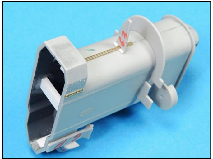
Note the tiny lengths of .015 x .015 inch strips to add strength to this long platform. Set all the vertical ladders with tiny drops of white glue first so they can be adjusted. Then add tiny drops of super glue between the ladder rungs.
