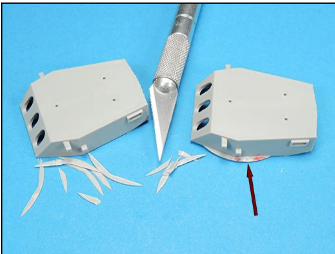
I used the tip of a number 11 X-Acto blade to carefully scribe the edges of the plastic. Several passes cut the plastic deep enough so it could be snapped off. The edges of the turrets were then sanded smooth.
