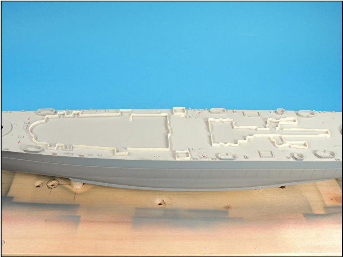
The hull was primed and then strips of masking tape were applied along the raised forward and aft superstructure positioning areas so that I would not have to scrape the paint off for gluing.
