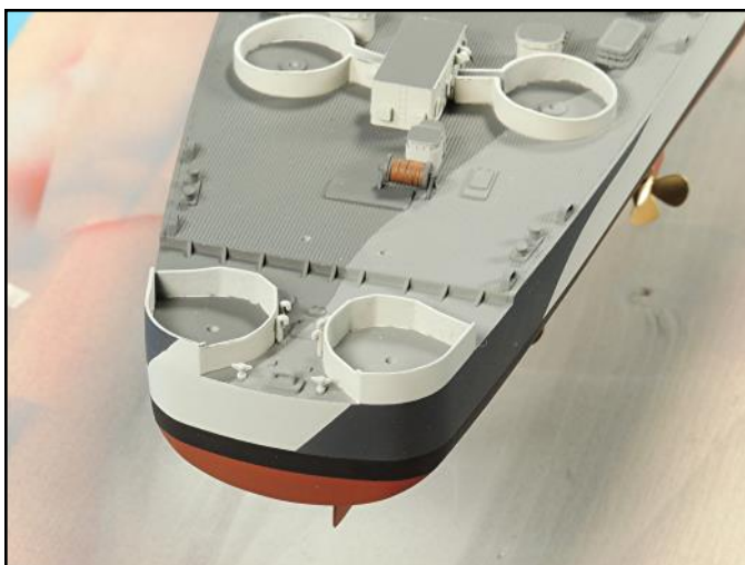
The tiny parts at the stern were attached with white glue so their positioning could be adjusted.
