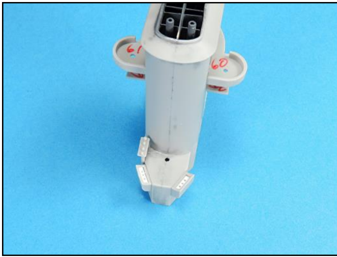
The flag boxes had .040 x .080 inch strips inserted with pre-drilled holes for the flag rigging. The inserts were attached with Testors tube glue.
