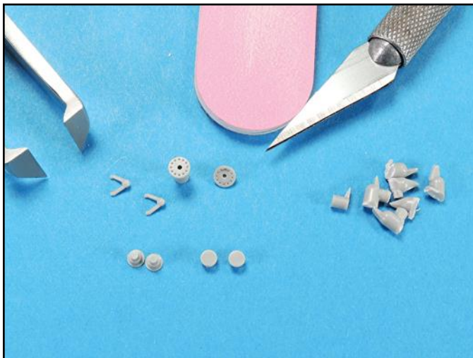
Small circular parts have to be carefully removed so as not to damage the shape of the parts. Trimming with the tip of a number 11 X-Acto blade and then light wet sanding of the surface is sometimes needed to restore the part's shape.
