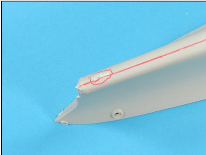
The other injection point is on the bow. Be careful not to distort the shape of the bow when you sand this one smooth. There is also a seam line that runs along the bottom of the hull. Carefully scrape this off and then wet sand the surface.
