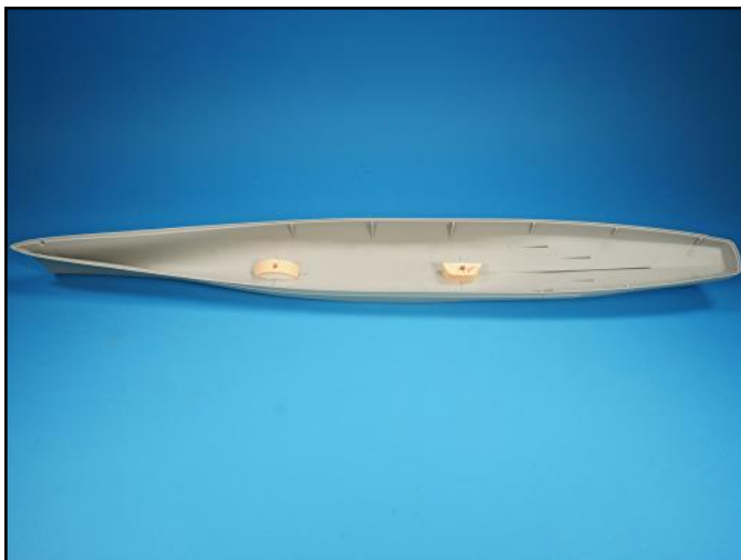
The brass display pedestals locations were marked and small holes were drilled through the hull. Blocks of resin were glued inside the hull at the hole locations so the pedestals would have a solid foundation for attachment and gluing.
