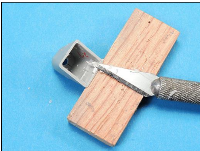
The insides of the pedestals along the seams were scraped flat so that tiny strips of plastic could be glued to strengthen the seam.
