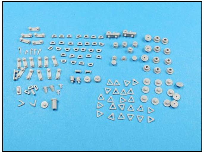
All the deck fittings have been cleaned up and they are now ready for assembly. Be sure to flatten the tops of the bits and the bottoms of both the bits and chocks so that they will sit flat on the deck.
