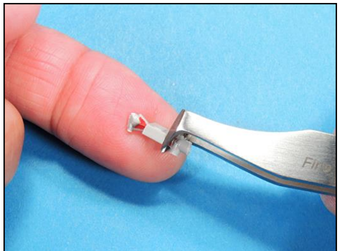
Here is an example of large tree attachment points on a small part. Here again the snippers work best for removing the plastic without damaging the part's surface.
