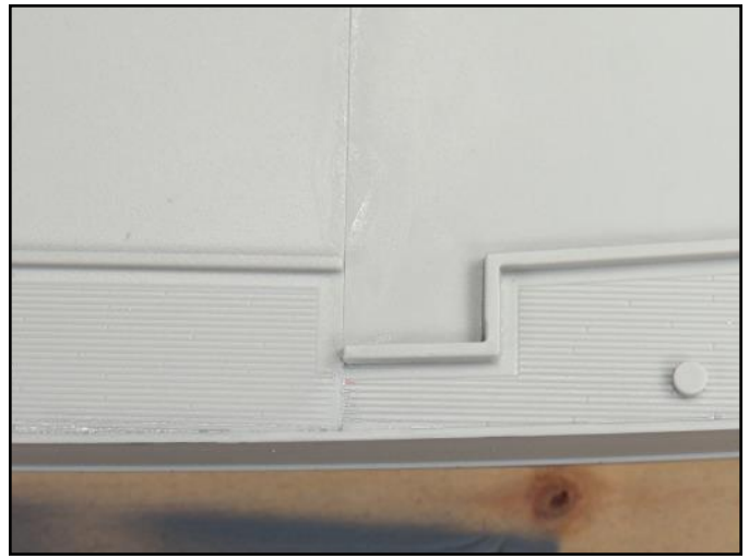
The deck seams had tiny drops of super glued added. The areas were then carefully scraped flat and wet sanded with 600 grit sandpaper wrapped around a piece of balsa wood.
