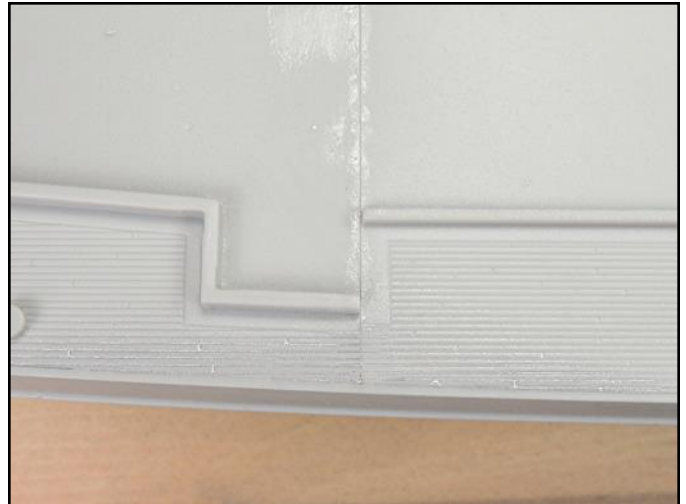
Once the deck is primed and painted you will have to use a magnifying glass to see were the deck detail was restored. The plastic is soft so use light pressure when re-scribing the deck detail.
