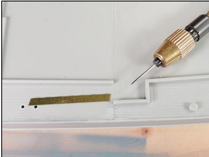
A sewing needle and length of photoetch brass were used to re-scribe the wood deck detail at the seam locations. Only two light passes were necessary to restore the deck detail.
