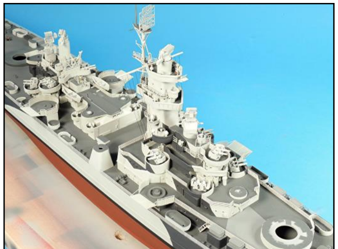
The angled cage railings for the forward 5 inch/38 platforms were attached and then the 40mm guns were added.
