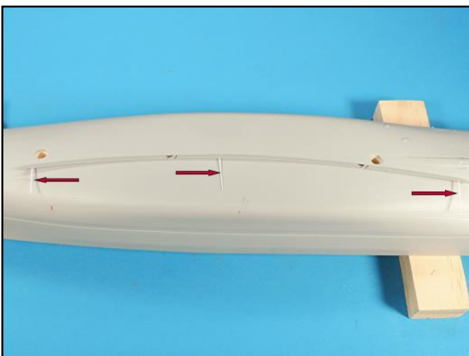
The side keels are separate parts and one was warped. To help set the keels into place I tried pinning them into place with .020 inch plastic rod. This did not work very well.
