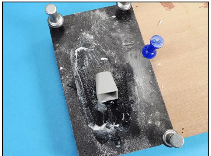
The backside of the vents and the sides of the catapult pedestals were run across wet stationary fine grit sandpaper to smooth out the super glue. The plastic was then polished with a 0000 steel wool pad.
