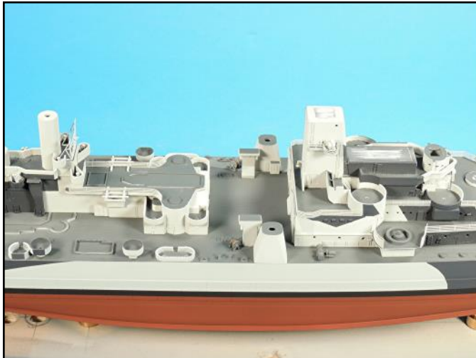
I then turned my attention to the aft superstructure and added the crane cradle and tower supports and then the railings.
