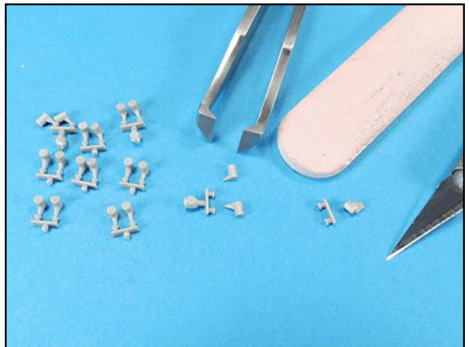
Slide molding can sometimes have a lot of plastic injection points on parts that are not attached to trees. Snippers are the best way to remove these free floating excess plastic points.
