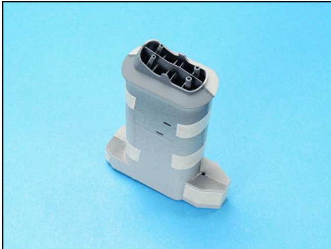
The stack was tightly taped together and then a bead of super glue was applied along the seam lines.
