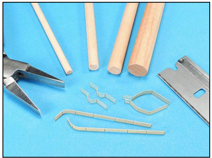
I used various size wood dowels to get the correct curves in the photoetch railings.
