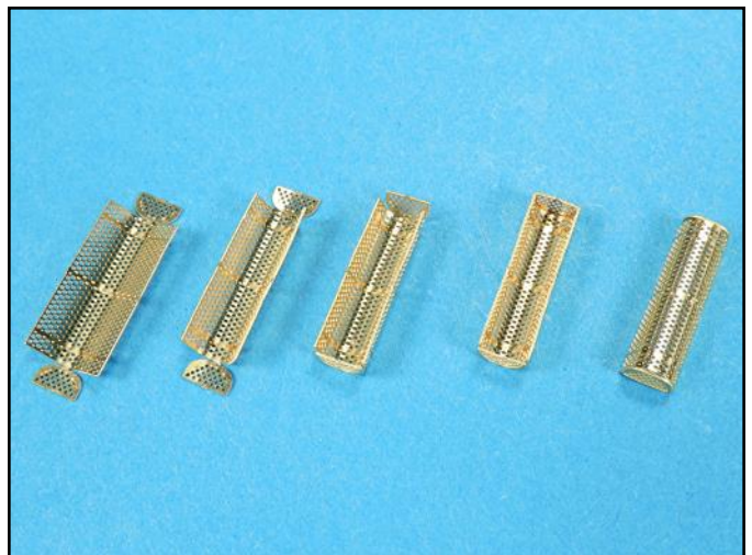
Here are the 4 stages for forming the round floater baskets.
