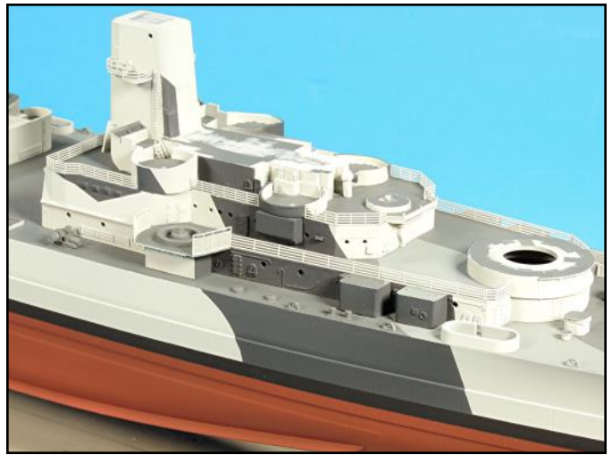
I added the forward superstructure railings first starting at the searchlight platforms and working my way down. I used white glue to set the railings in place and then applied a tiny bead of super glue along the base of each railing.
