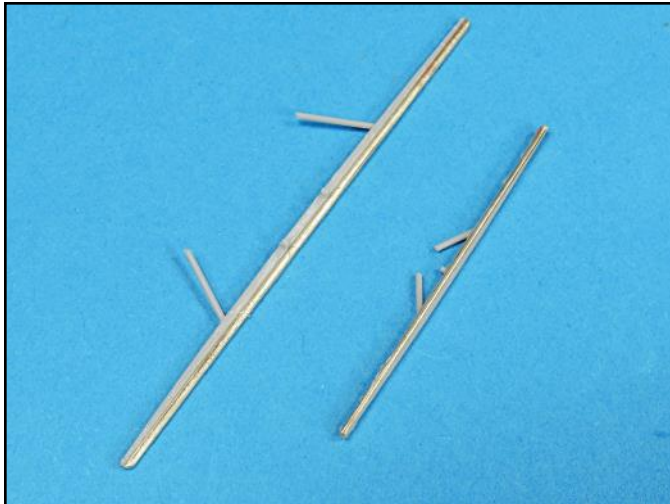
The forward and aft yardarms were reinforced with stiff .028 inch brass rod that had one side flattened by running them across sandpaper.
