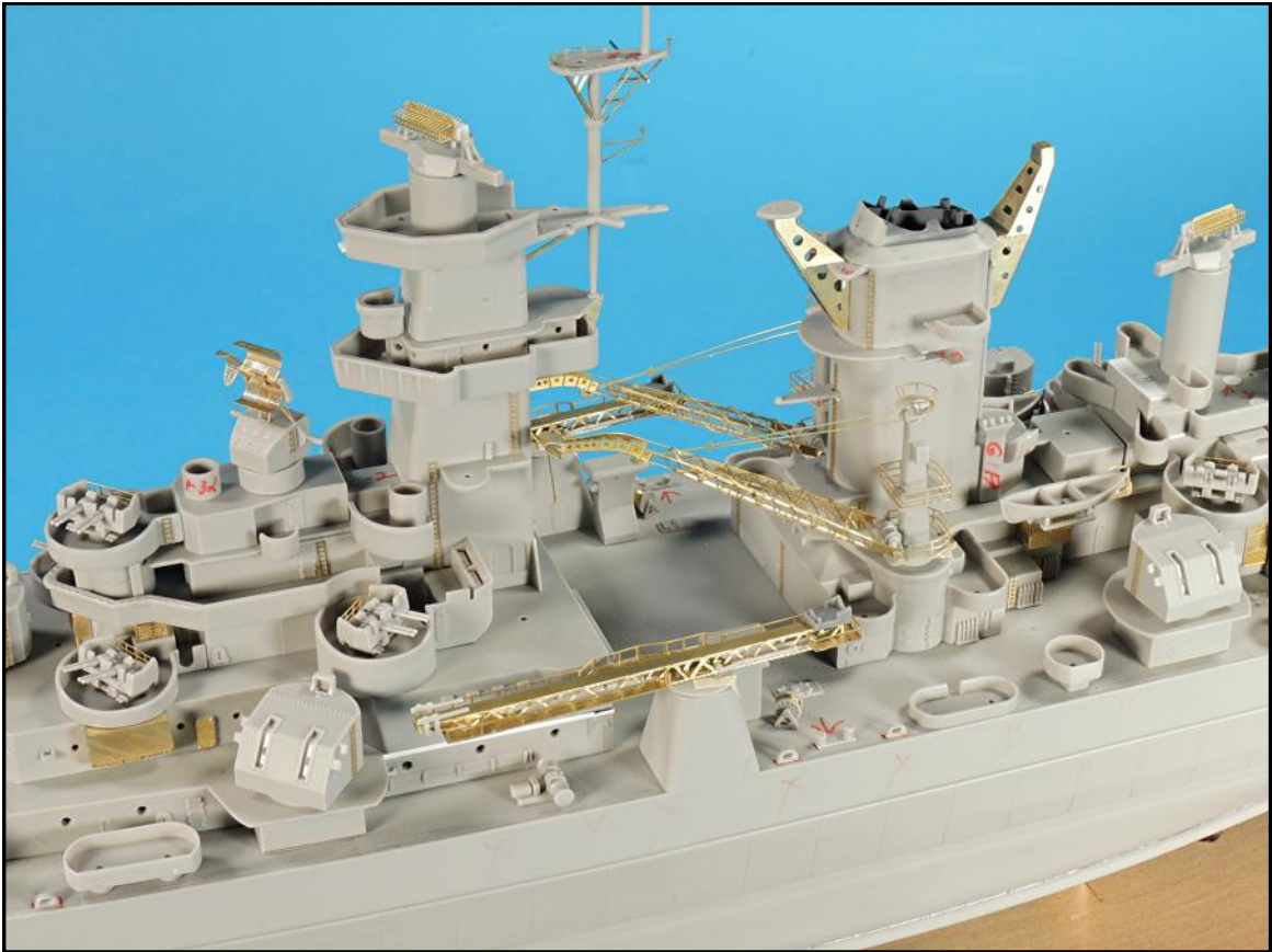
The catapults and cranes are off balance so they will need to be attached with Testors tube glue.
