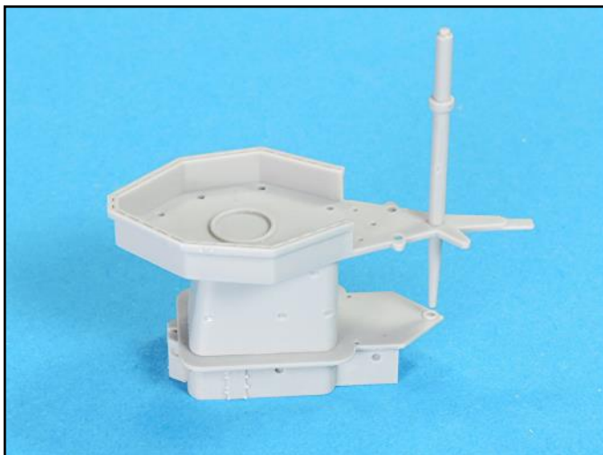
The main mast positioning hole needed to be drilled out with a .070 inch bitt to that the mast would sit correctly.
