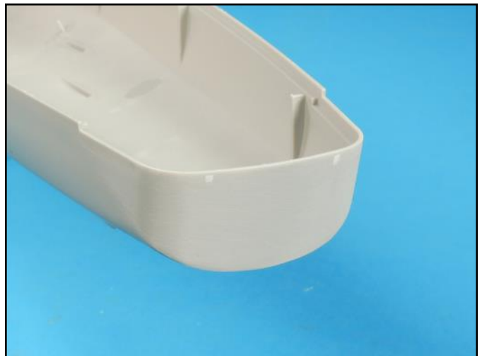
The stern area has been sanded smooth and polished with 0000 steel wool pad.
