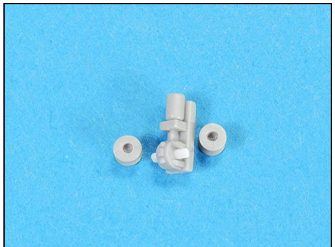
The rod was glued into place with tiny drops of super glue and then trimmed. The windless reels were carefully drilled out using a .025 inch bitt and then a .037 inch drill bitt.
