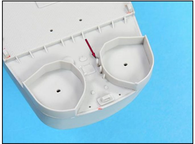
The holes for the vents at the stern also need to be slightly enlarged for a better fit. These were drilled out with a .025 inch drill bitt.
