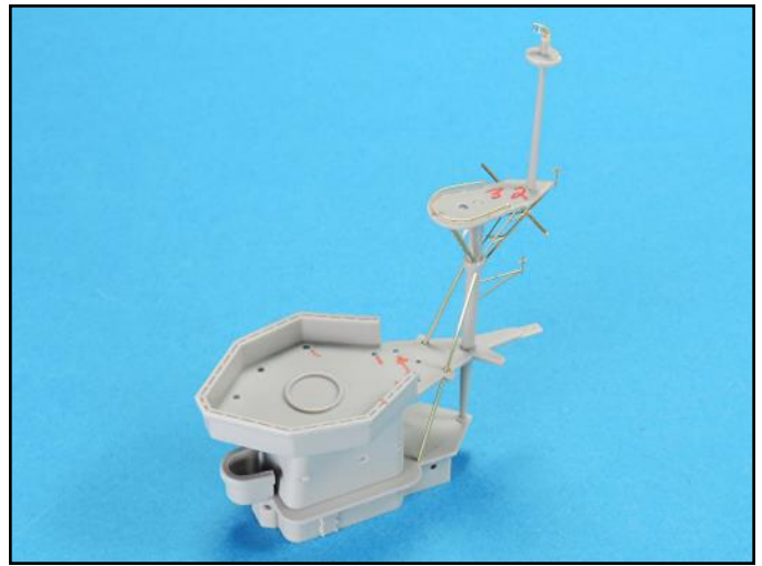
The kits plastic mast support braces were also replaced with .019 inch brass rod.
