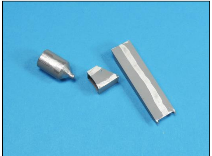
Always check seams with Testors silver paint as it will highlight flaws. Apply more super glue to any identified flaws and then sand smooth.
