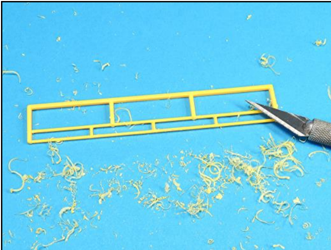
The railings have heavy mold lines that need to be scrapped off using a number 11 X-Acto blade. Hold the blade at approximately a 45 degree angle and carefully and lightly scrape off the mold lines.
