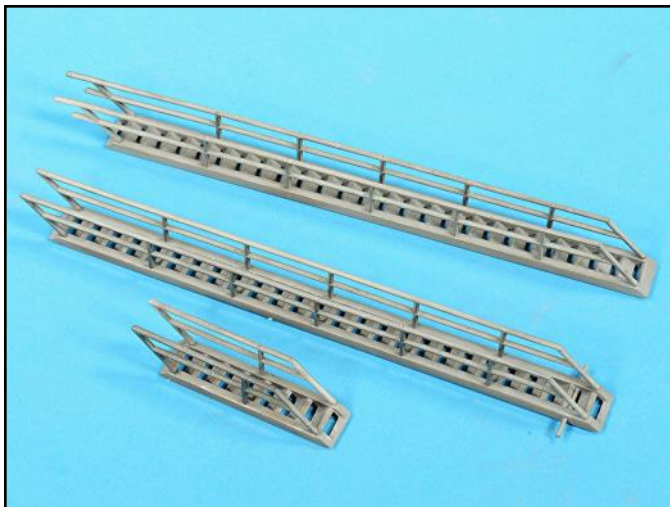
All the railings are installed and these assemblies are ready to be attached to their platforms.
