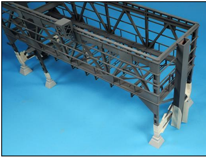
Areas around the foundations were also masked to protect them from overspray.
