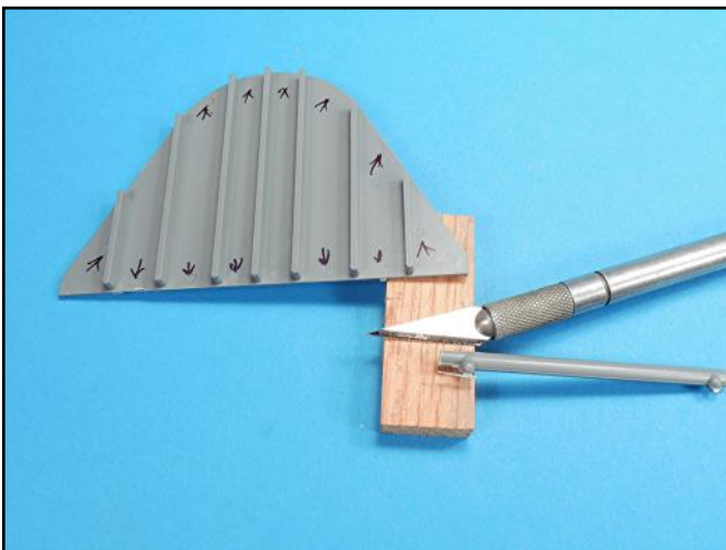
I decided to cut the stub with a number 11 X-Acto blade on an elevated wood block and that approach did not damage the parts edge.
