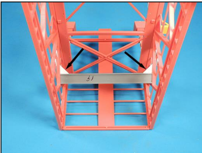
The bin has been removed and triangle shaped support plates were added to the girder to strengthen the assembly.
