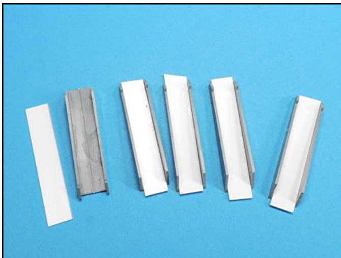
The inside seam needed to be hidden so strips of .015 inch thick plastic strips were laminated to the inside area. Each strip was approximately 3/8 inches wide.
