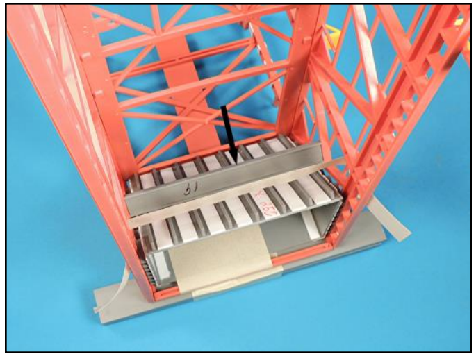
The smaller coal bin was positioned inside the structure and taped into place. The support girder was then positioned and glued into place.
