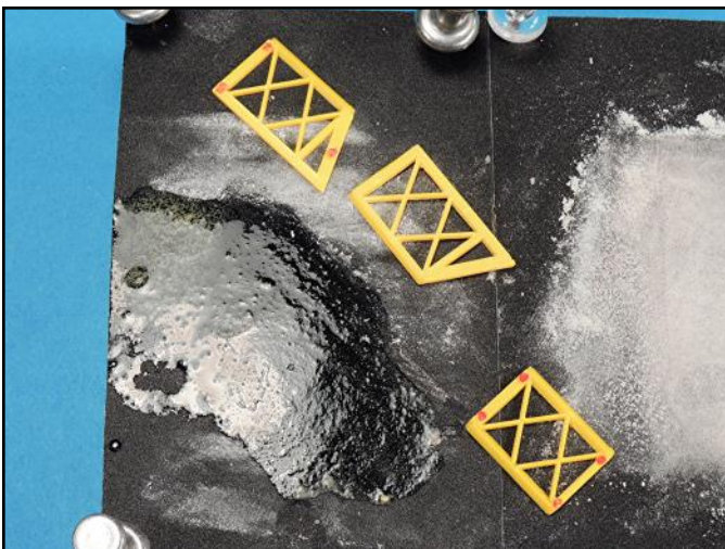
There were mold punch outs on the surfaces of the upper level stairway platform. They were removed by running the parts across a wet stationary piece of fine grit sandpaper.
