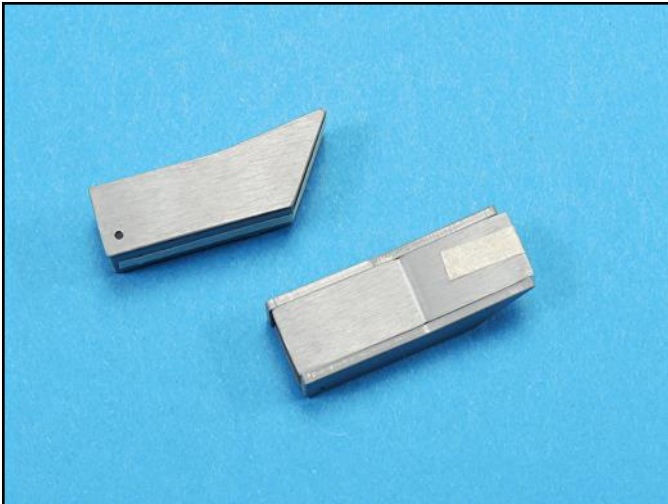
These chutes were also taped together, super glue applied along the seam lines and then the seams were carefully scrapped and sanded smooth.
