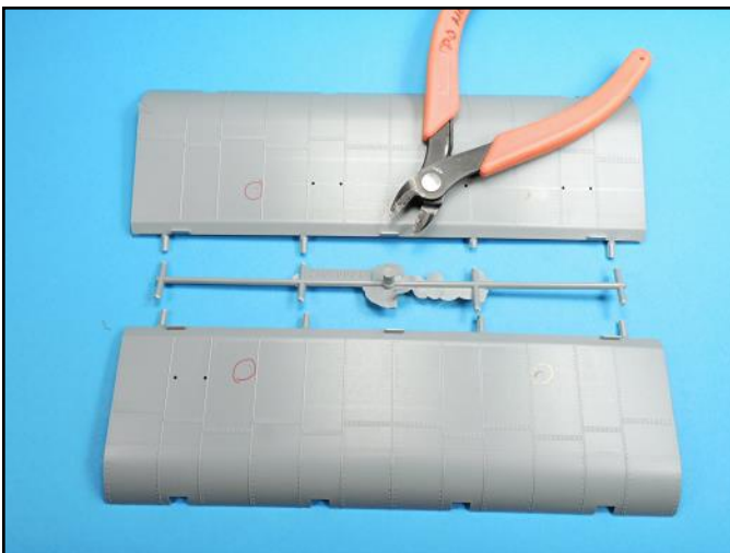
These tree attachment points were very thick and were cut with plastic cutters. The remaining tree stubs can now be carefully removed without damaging the edges of the part where they were attached.
