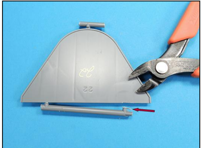
Using a cutter to separate the stub from the part resulted in damaging the edge of the part.
