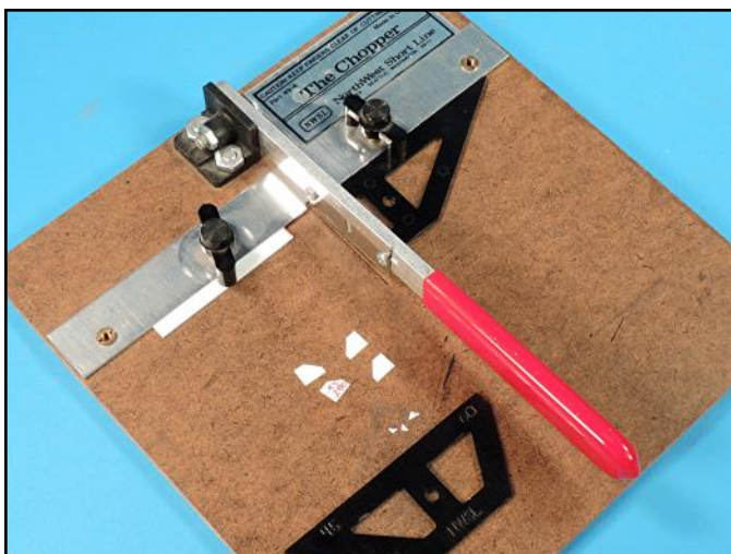
I made gusset plates from .015 x .250 inch strips for the base of the girder structure with my trusty chopper
