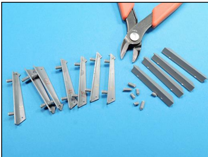
The coal chute parts were removed from the trees with some of their stubs left on the parts. The remaining stubs were removed and the surfaces carefully scraped flat.
