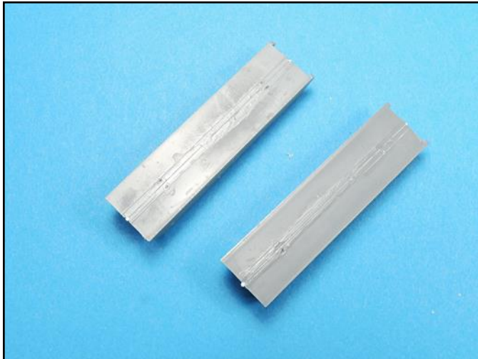
The chutes are now ready for the seam removal process.
