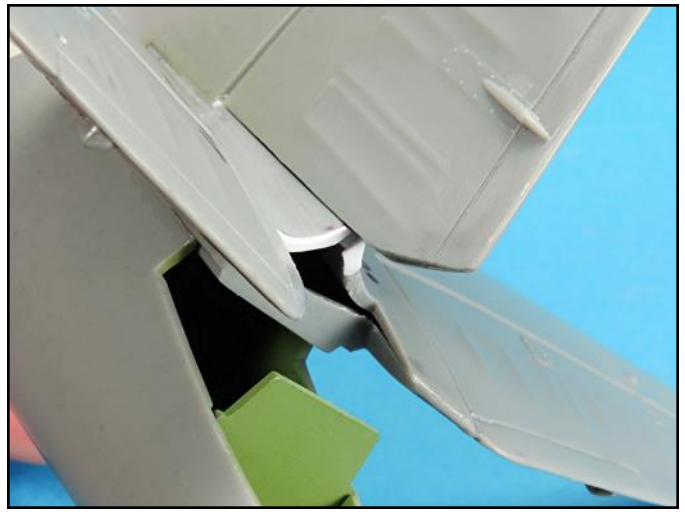
These tiny strips were added to help close up the void between this area and the aft clear part.
