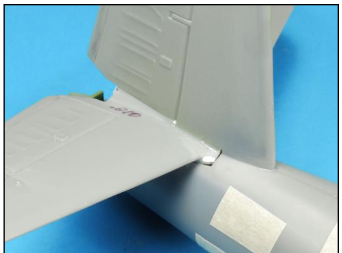
The tiny voids around the elevator assembly on the right side will have to be filled and shaped.
