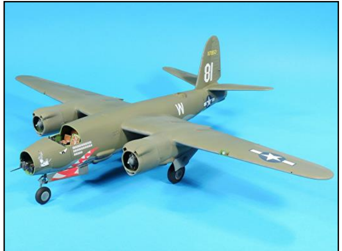
The engine cowlings were glued into place with slow set super glue.
