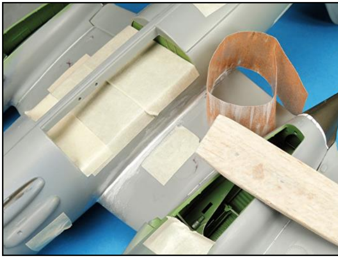
Note how the balsa strip ends are shaped so that the wet sandpaper can get into the tight area between the fuselage and the engine nacelle.
