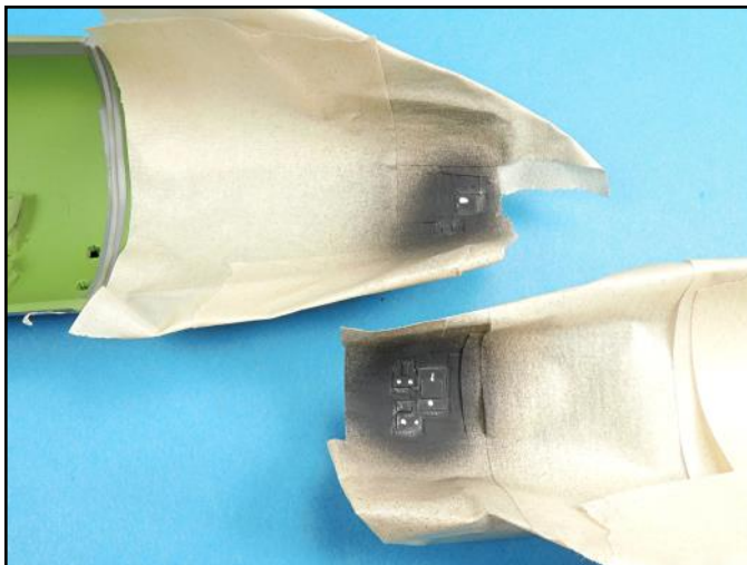
The electronics boxes were airbrushed flat black and the surface details picked out with flat white. The flat white paint was applied with the tip of a round toothpick.
