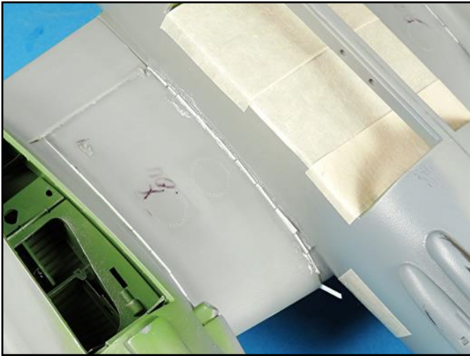
The underside on the left wing had its entire void filled with .015 inch thick strips. Super glue was applied to both sides to seal the areas around the strips and the tiny voids between them.
