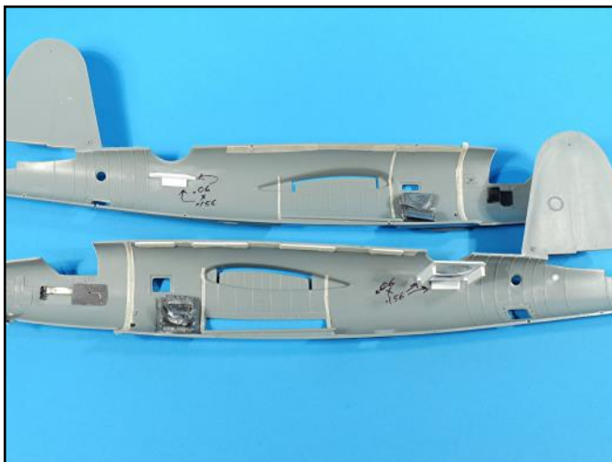
The fuselage interiors were masked in areas where parts would be glued into place.
