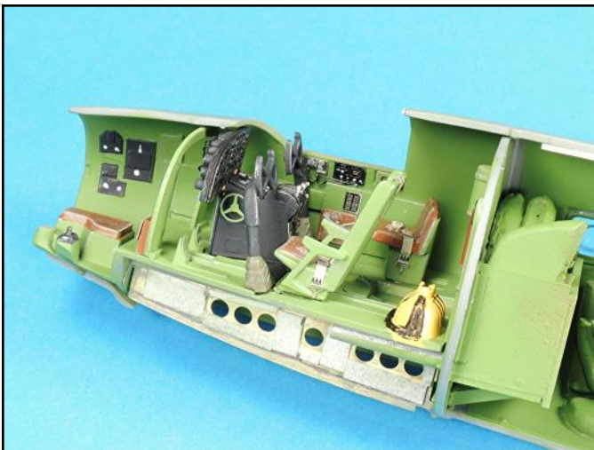
The trim wheel was added to the side of the console and then the cockpit assembly was glued into place.
