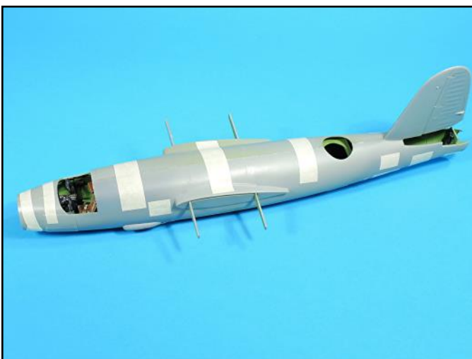
The fuselage halves were positioned with masking tape and beads of super glue applied along the seam lines.
