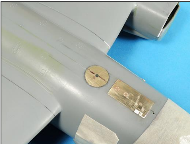
The perimeter of the round hatch also received a tiny bead of super glue.
