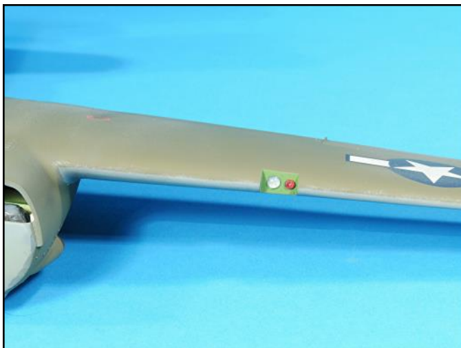
The leading edge wing lights has their backings painted silver and red. They were attached with tiny drops of white glue.
