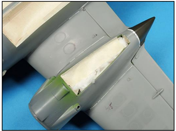
Tissue was stuffed inside the opening and then strips of masking tape were applied along the straight edges. Additional tape was then applied over the tissue to completely seal the openings.
