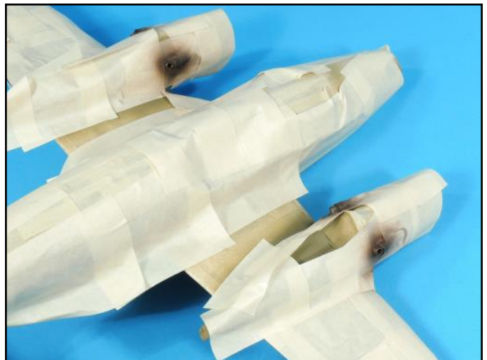
The engine exhausts were masked off and airbrushed with Testors burnt umber color.
