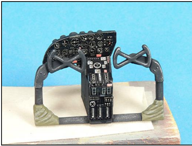
The Eduard pre-painted photoetch parts were attached using slow set super glue so that they could be properly positioned. The slow set glue provides about 5 to 10 seconds of working time before it dries.
