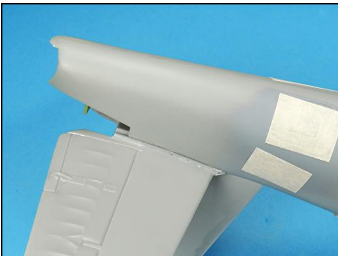
The underside seams on both sides of the elevator assembly were not bad so they were filled with super glue.
