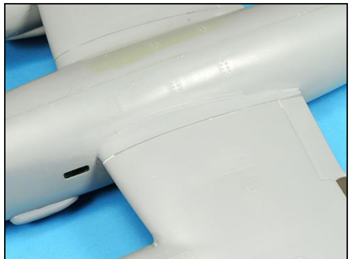
It took some time to get the step smoothed out and the surface contoured on the left wing, but the seam and the area around it look good.
