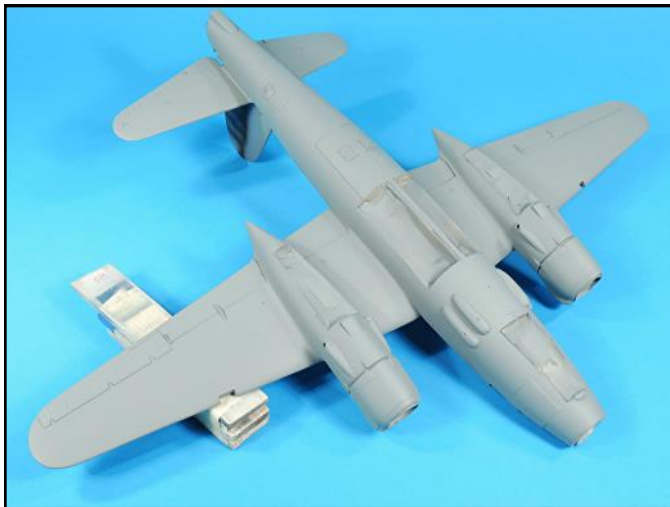
The lower surfaces were airbrushed with Testors dark gull gray.
