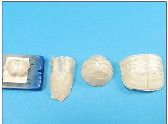
The clear parts were carefully masked with tiny strips of masking tape. The framing on the clear parts is very subtle, and the edges have almost no depth. This makes masking around them a challenge.
