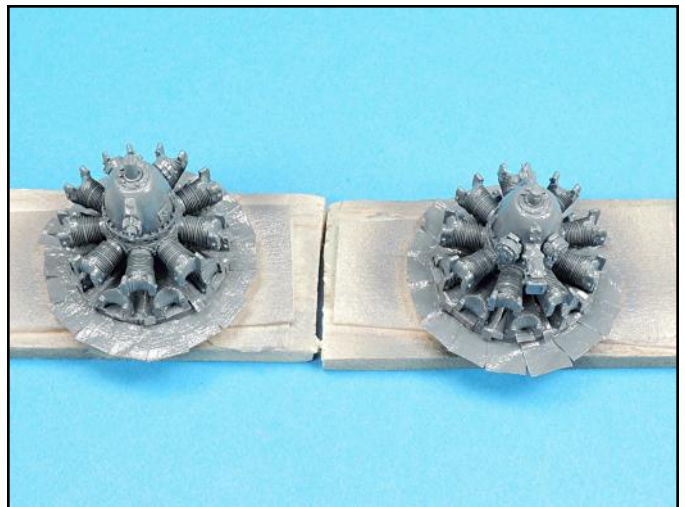
The engines were airbrushed with a gloss medium gray color.
