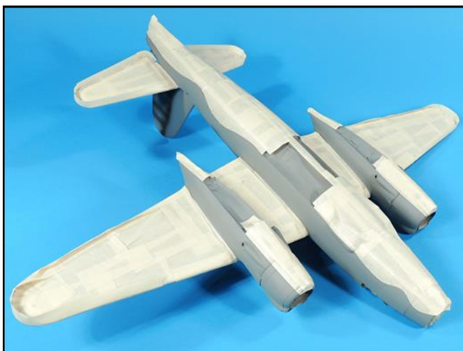
The entire lower surface area was then covered with larger strips of masking tape. Note the tape on the cowlings and the engine nacelles.
