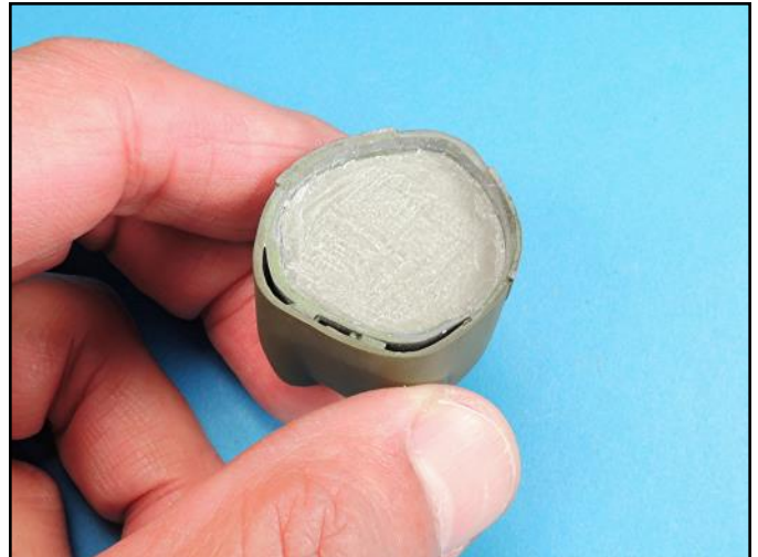
The right cowling would not sit flush against its engine nacelle, so additional resin material had to be carefully scraped off the engine backing until the assembly fit correctly.
