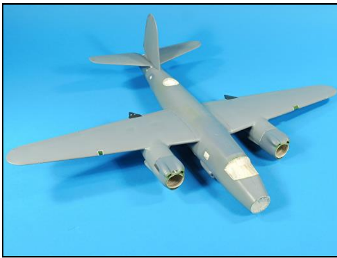
The insides of the engine cowlings were masked and then they were taped into place from the inside. The assembly was then primed.
