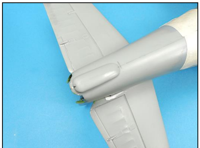
The tail skid was glue into place with Testors red tube glue so that it could be positioned. Note the pencil marks to help center the part.
