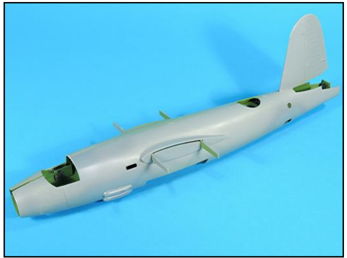
There is a slight misalignment between the left and right fuselage halves. I chose to have the bottom of the fuselage halves line up and then sand and shape the upper surface.
