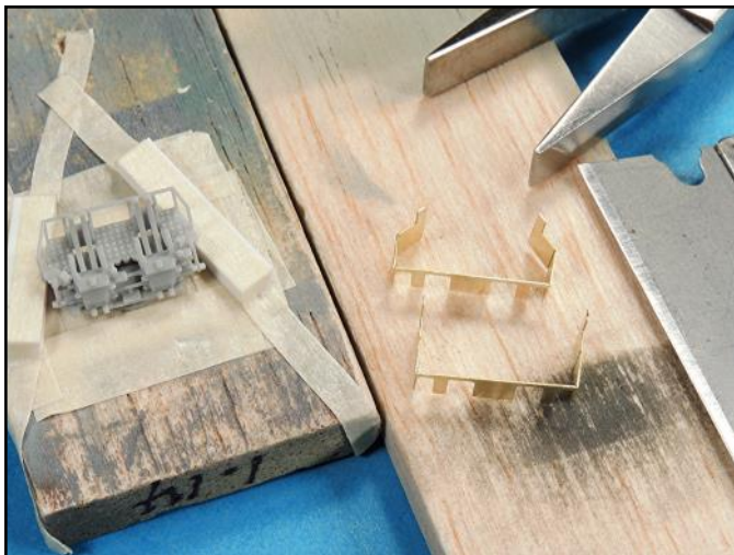
The photoetch splinter shields are easy to shape and the back sides have etched fold lines.
