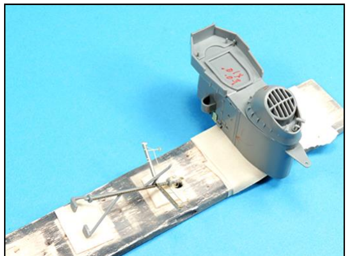
Using balsa strips and masking tape folded over itself is a great way to attach parts for airbrushing.
