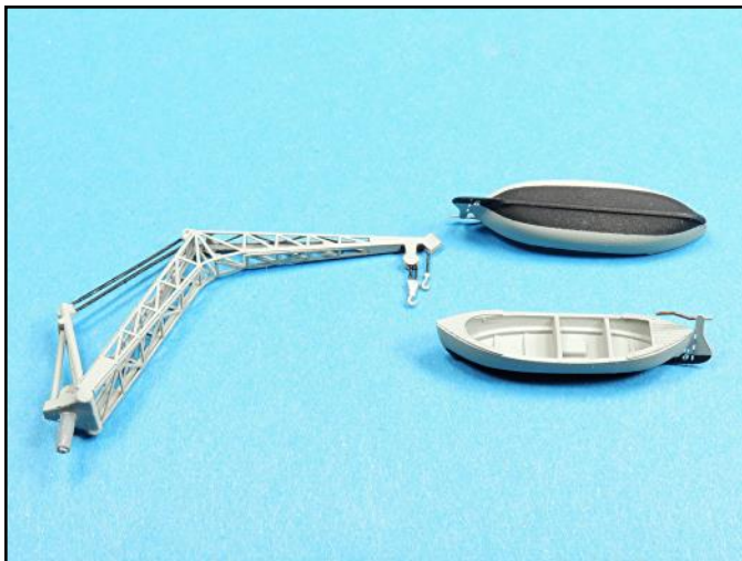
The whale boat propellers were painted brass and the tiller handles were painted leather. The cables on the crane were painted flat black and the hooks were painted brass.
