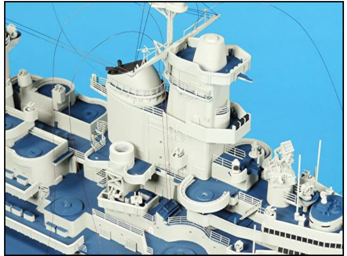
The nylon thread for the signal flag lines was inked with a brown indelible marker. Each length was threaded through its corresponding hole in the yardarm and down to its location in the signal box and then glued into place.
