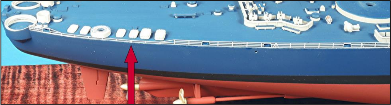
The short stern deck railing has been installed.
