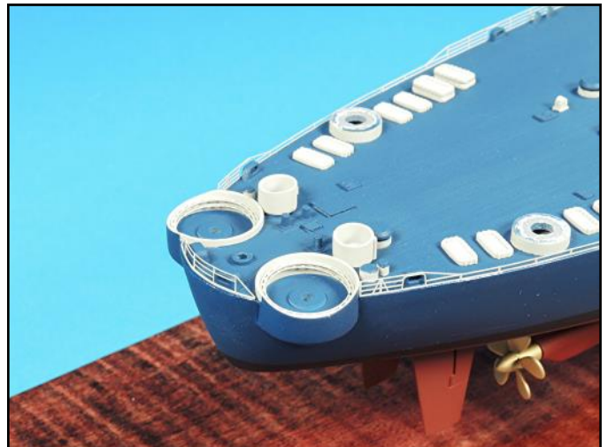
The Eduard stern railing was used because I bent the Gold Medal Models railing. All the railing bases on both sides received an airbrushed coat of Testors dullcoat at 15psi to hide the super glue.
