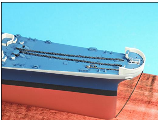
The bow 20mm platform was attached and the tiny seam along the attachment point to the hull was filled with white glue, contoured with a damp Q-Tip and then painted with flat gull gray with a detail brush.
