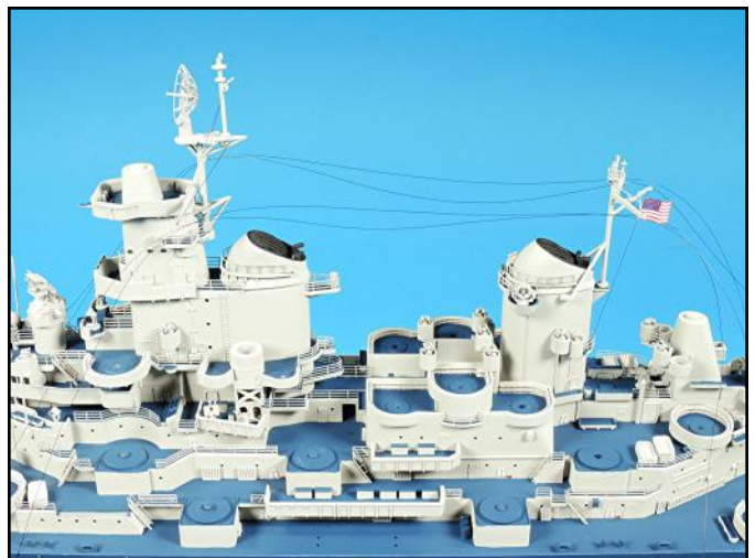
The rigging between the forward and aft masts was installed using nylon thread inked black. The rigging was carefully threaded through the tiny photoetch rings on the mast yardarms.
