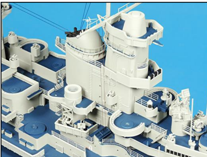
Always start installing signal flag lines from the inside towards the outside. Install one or two at a time on both sides and work your way out to the last one.
