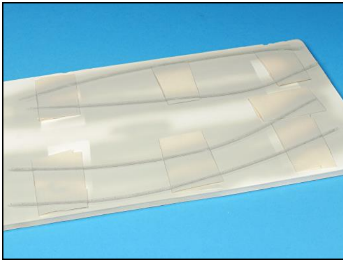
Long, straight railing lengths can be airbrushed by slightly curving them while attaching them to masking tape. This prevents them from falling over while being airbrushed.
