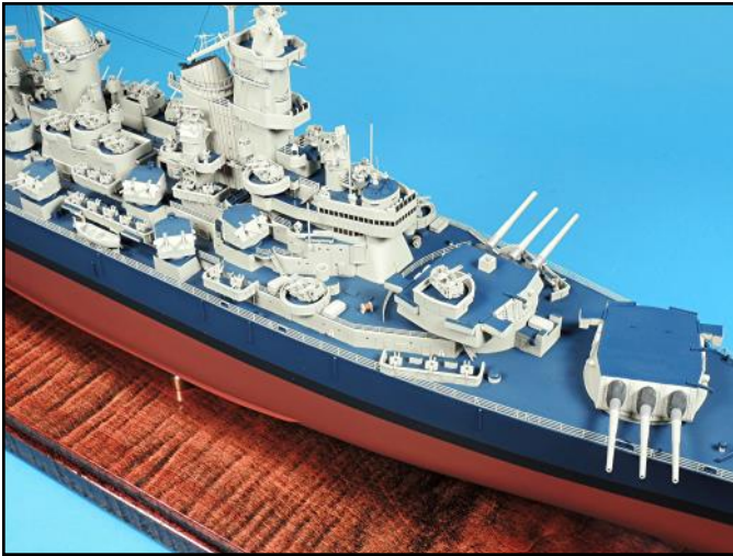
The 16 inch turrets, 40mm Bofors and Mk-51 directors have been installed along with main deck 20mm guns.
