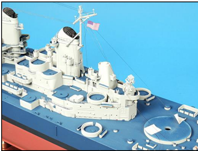
The aft signal flag rigging was installed through the tiny photoetch rings on the yardarm and held taught with masking tape until the glue dried.
