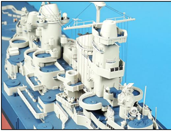
All five signal flag lines are installed on both sides.
