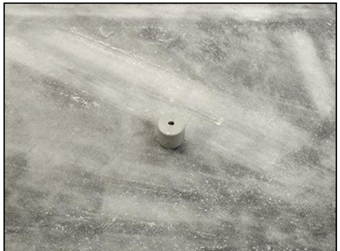
The radar platform bases and tops were flattened by running them gently across a stationary piece of sandpaper.
