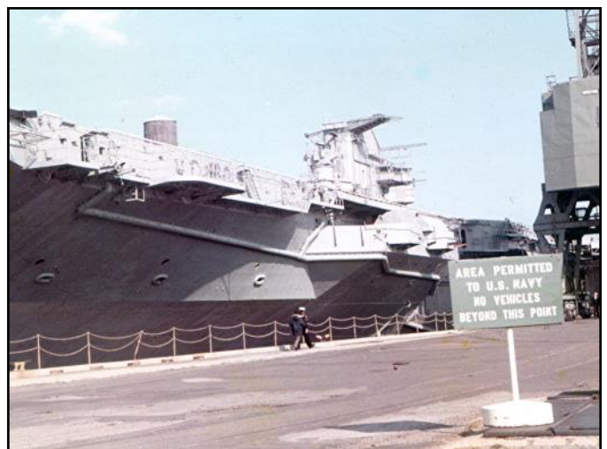
Note the external hull piping. While not the same as it was configured during WW-II, it is very noticeable and that is why it is necessary to add these hull details to the model.
