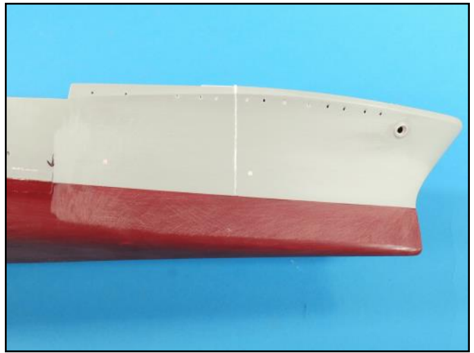
The initial sanding smoothed out the plastic strips and the flat area on the upper hull was also reshaped.
