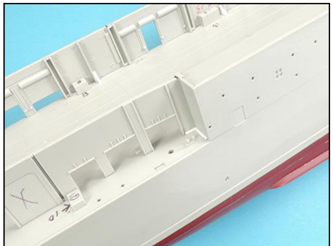
The inner corner at this location would have been impossible to fill and sand smooth. Careful cutting and form fitting of .030 inch quarter round fixed the problem.
