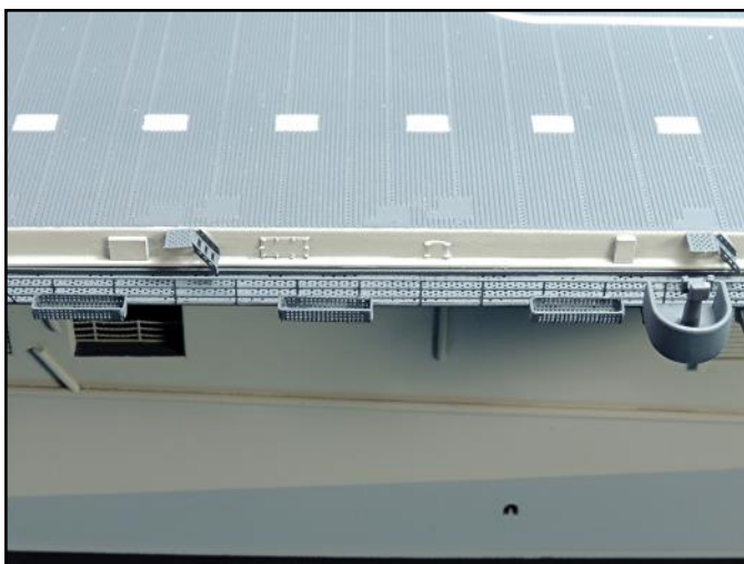
The flight deck catwalks were airbrushed and then attached to the sides of the flight deck with white glue. The edges of the catwalks fit snugly and tightly into the channels. The floater net cages were then white glued to the railings.
