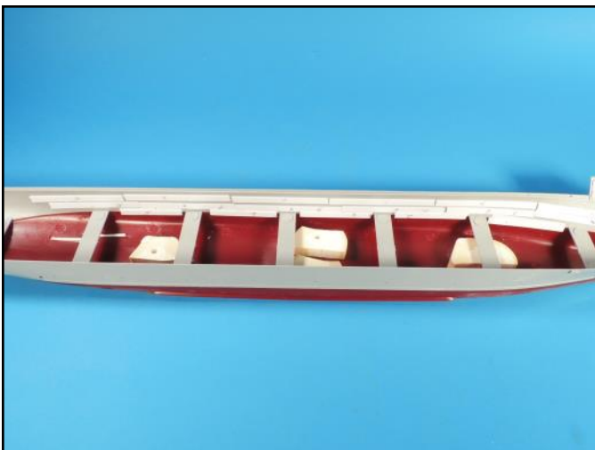
The same reinforcement strips that were laminated to the interior of the Franklin's hull were also added to the long hull.
