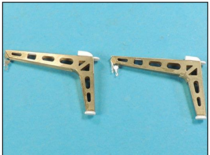
The raised disks on the hanger deck for the cranes were damaged during sanding the hanger deck seam line. New disks were added to the crane bases using a Waldron punch tool. This made the cranes fit tightly into their locations.
