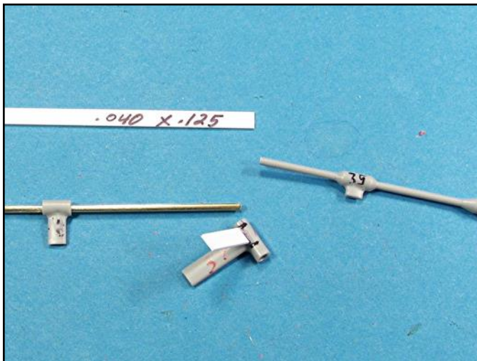
Now that the outer strut can be rotated, add .04 x .125 inch strips for the additional legs on each of the four outer "V" struts. There is a reference photo on page 64 that shows the stern of the Essex class carrier Yorktown in dry dock.
