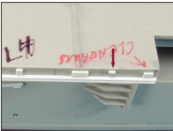
Tiny positioning tabs were added to the sides of the flight deck to provide a positive attachment point for the small inclined steps.
