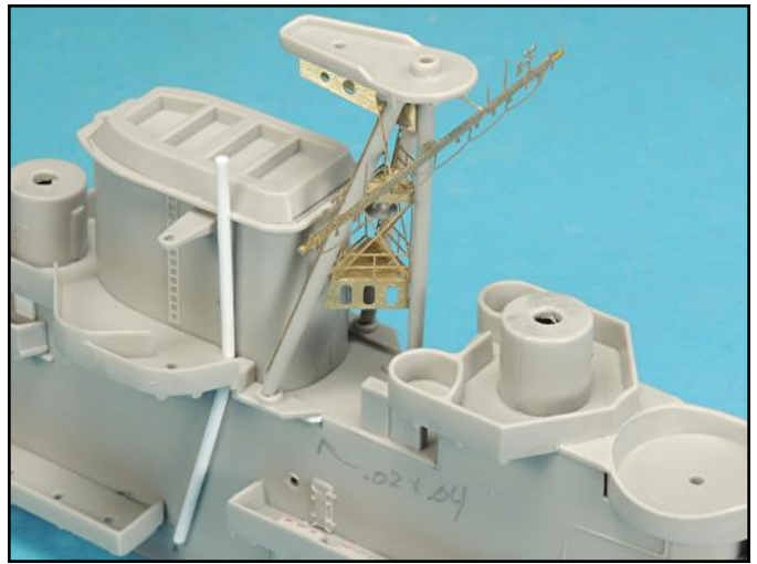
One last fit check of the tripod assembly was made to be sure that the legs fit into their locator holes on the deck correctly.
