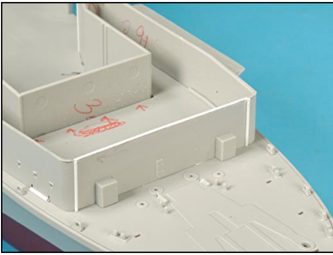
The forward superstructure needed some plastic strips added to fill the voids between the upper edges and the underside of the flight deck.
