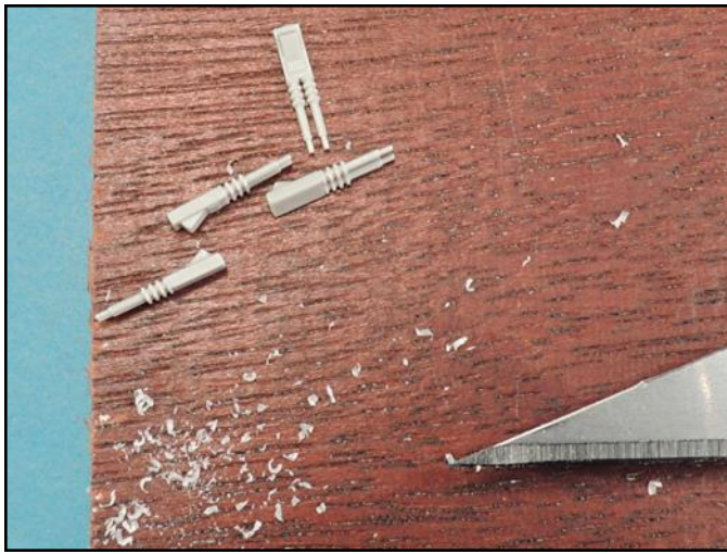
To remove the mold lines from the outer edges of the guns, carefully scrape the excess plastic off using a number 11 X-Acto blade held at a 45 degree angle.
