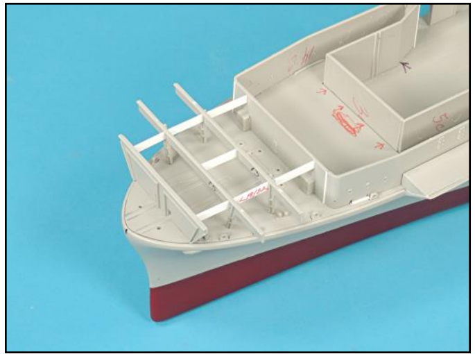
The forward sea shield was set in place and then additional cross framing was added. This additional underside framing can be clearly seen in reference photos. This also made the assembly very sturdy.
