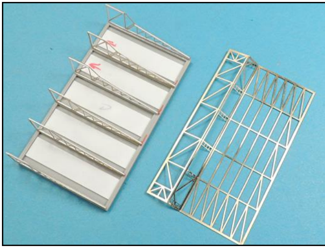
The inter framing was added and the bottom framing was then checked and adjustments were made to its shape by adding more bend to the fold lines using a sewing ruler.
