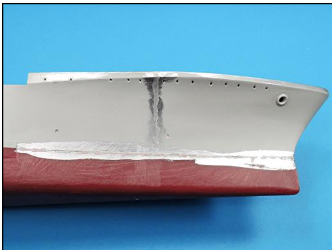
Almost the entire seam line on the both sides of the hull needed several additional applications of super glue.
