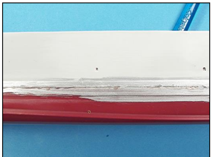
The hull seam line was carefully wet sanded smooth by wrapping sandpaper around a section of balsa wood. Silver paint was applied to check for flaws and more super glue applied along the seam line.
