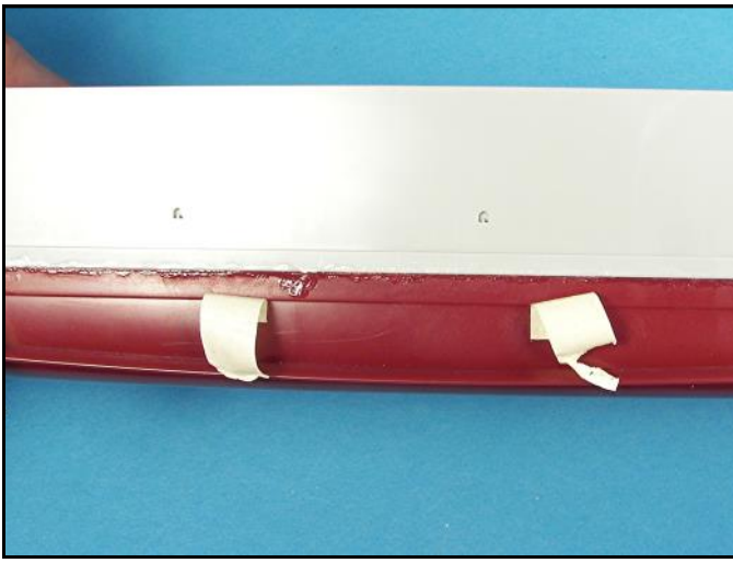
The tape was removed and super glue was applied to these area.
