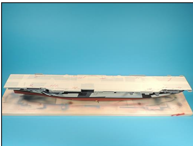
The flight deck was positioned on the hull so the dazzle pattern color locations could be transferred to the flight deck platform splinter shield outer surfaces.
