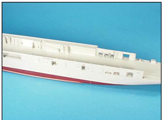
As each section is added, work on the seams. This is a much better approach than waiting until everything was glued into place. That much seam work at one time can be overwhelming.
