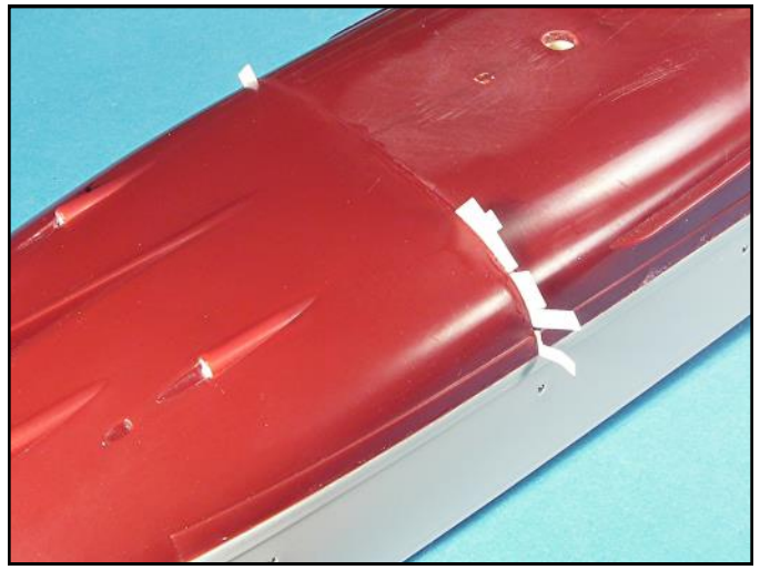
The cut lower hull section was positioned and glued into place. Strips of plastic of various thicknesses were used to fill the gap. Super glue was applied to both side of the strips and in between them.
