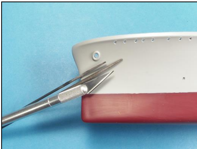
The port holes were drilled out using a .046 inch bit. The anchor holes were drilled out with a .086 bit and then carefully shaped with files and the tip of a number 11 X-Acto blade.
