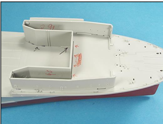
The outer parts and the superstructure side have been glued into place. Note the gaps at the base of the forward superstructure sides.
