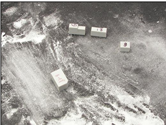
Some parts had uneven bases that need to be corrected. Run these parts across a stationary piece of wet sandpaper. Check your work as you progress to be sure the parts will sit level.
