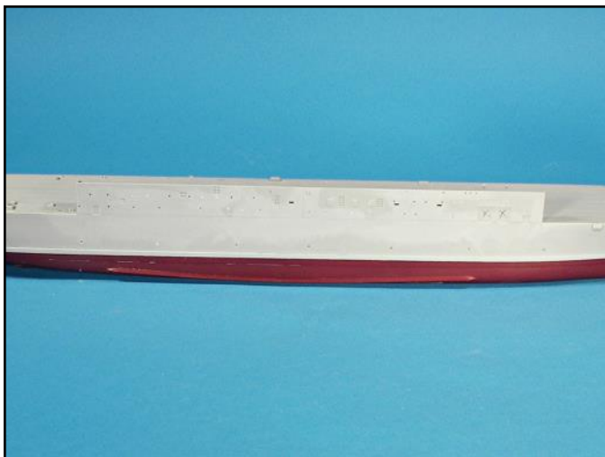
The starboard side sections that were attached first are flush with the hull so the seams were filled with super glue and the surface sanded smooth and then polished with 0000 steel wool pads.
