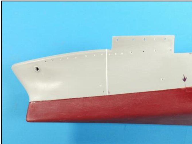
The port side only needed to have the plastic strips flattened out. The seam lines between the upper and lower hull were also sanded smooth.
