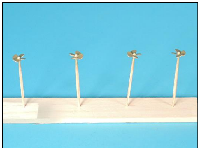
To make sure the propellers are not mixed up etch numbers 1-4 on the backside of one of the blades on each propeller and note these numbers on the instructions. The propellers were airbrushed Testors brass color.
