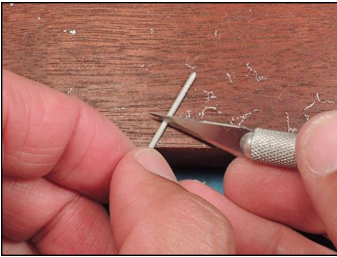
Scraping the seam lines on the island superstructure tower legs was done very slowly and lightly so as not to distort the round shape of the legs.
