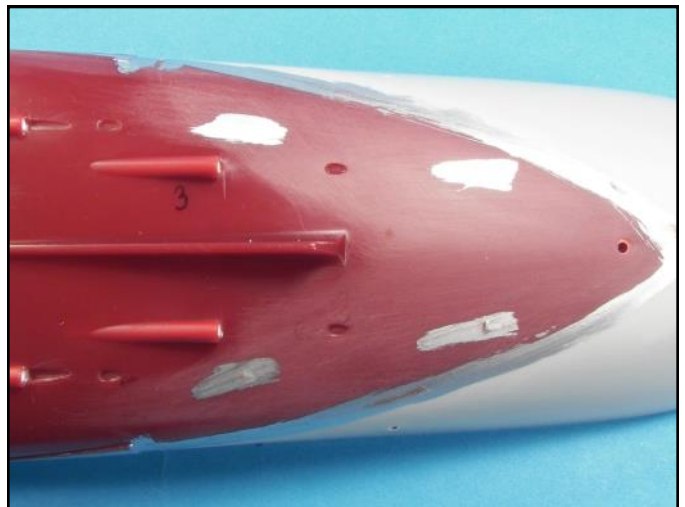
The indentations in the lower hull for the propeller shaft struts were filled in with small sections of strips plastic, super glued into place and sanded smooth.
