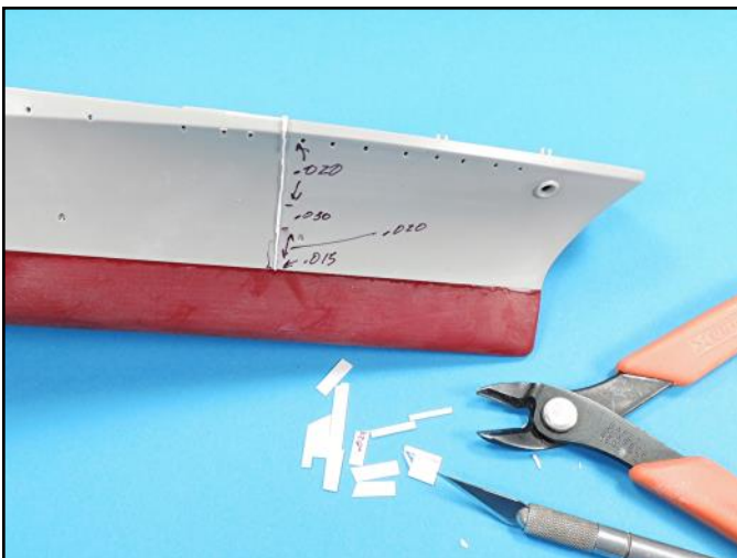
The starboard side was trimmed before the port side was worked on. As the repositioning, rechecking and adjusting was done, the original openings size on each side of the hull were reduced slightly.
