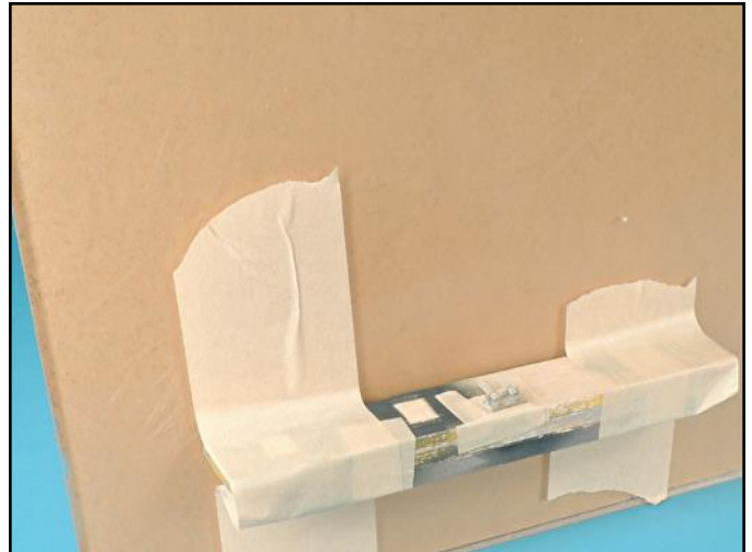
An easy way to set the back railing on the 40mm gun platforms is to position the assembly vertically and then attach the railing.
