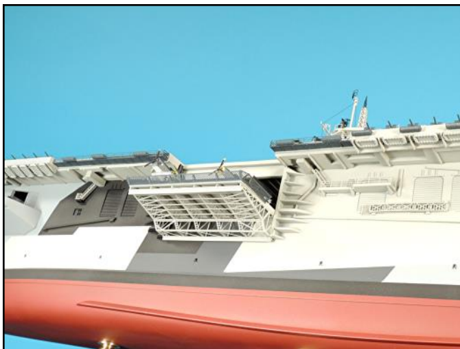
Small sections of plastic were painted and then glued into place on the underside of the flight deck so that inclined ladders could be attached from the platforms to these added strips. This detail was missing from the kit.
