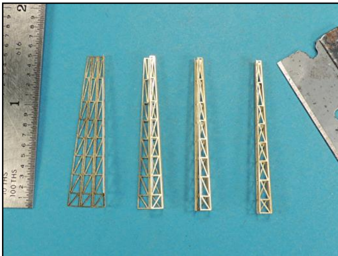
A sewing ruler and a single edge blade were used to fold the antenna towers.
