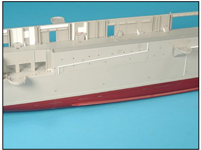
Additional fuel drain lines were also added to the aft starboard side of the hull. Note the small angle supports that were added to the inside areas of the superstructure sides to add strength.
