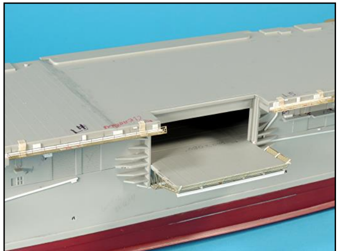
The catwalks and the side elevator are getting a fit check. The catwalks fit tight inside the channel shapes added to the sides of the flight deck. Once everything is painted, the channel shapes will be hard to notice.
