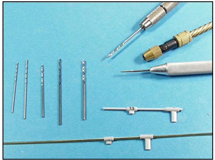
The kit's propeller shafts did not have "V" struts. The first step was to cut off the plastic shafts and drill holes through the struts for .052 diameter rod. The struts were drilled out to .058 inch diameter so there would be wiggle room.
