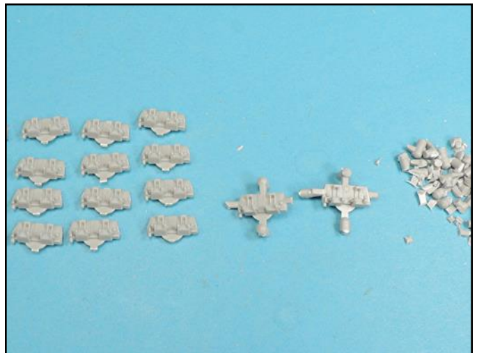
The kit's 40 mm gun bases had 4 tree attachment points and each one was very thick. Be careful how you remove the stubs from each part, as the edges can easily be damaged.
