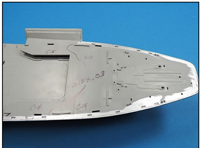
The seam line between the deck edge and the hull also need more super glue.
