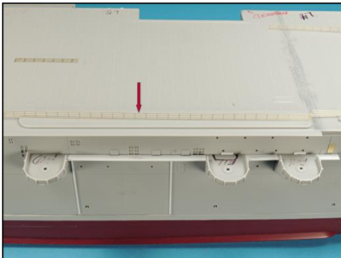
The railing length located on the starboard side next to the island superstructure is a long section with small bends in it.
