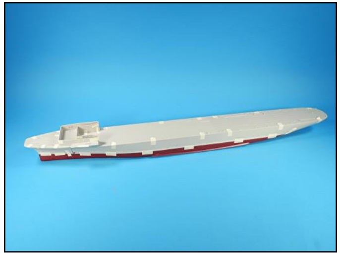
As the fitting, taping and adjustments continue, the forward upper deck is taped into place along with its associated superstructure. The superstructure ensures that the deck will be aligned correctly with the hanger deck.
