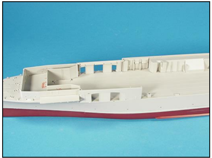
Hanger deck superstructure parts were attached starting at the forward area. Each section was carefully positioned and then beads of super glue were applied along their vertical and horizontal attachment points.
