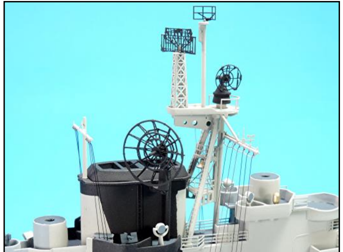
Note the clean appearance of the radars. The searchlight had to be repositioned because it was knocked slightly when attaching the radars. The yardarm rigging for the signal flags was inked with a brown sharpie marker.
