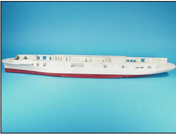
The fit check of all the hanger deck superstructure parts indicated that there were some fit issues at the aft end. Gluing all the other parts in place first helped determine what remaining aft end parts needed to be modified.
