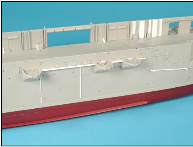
Reference documentation showed drain lines on the starboard side. These were added with .030 inch rod.
