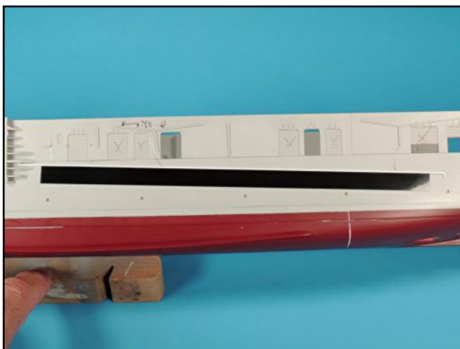
There was a lot of exterior hull piping detail that was missing from the kit. Using the ship's drawings, pencil lines were drawn for all the external piping locations on the hull. Labeling tape was used to set the piping lengths straight.
