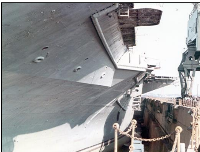
Looking down the port side of the hull, there is no noticeable torpedo belt. Either it was removed sometime after WW-II or the ship never had one.
