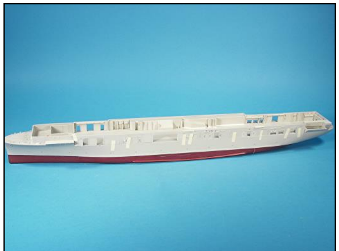
After all the roller doors were removed, the superstructure parts were re-taped together to determine if any other doors needed to be removed. With the side elevator roller doors completely removed the part had a slight upward curve to it.
