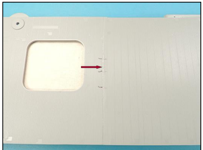
The seam line on the aft flight deck was a very tight fit.
