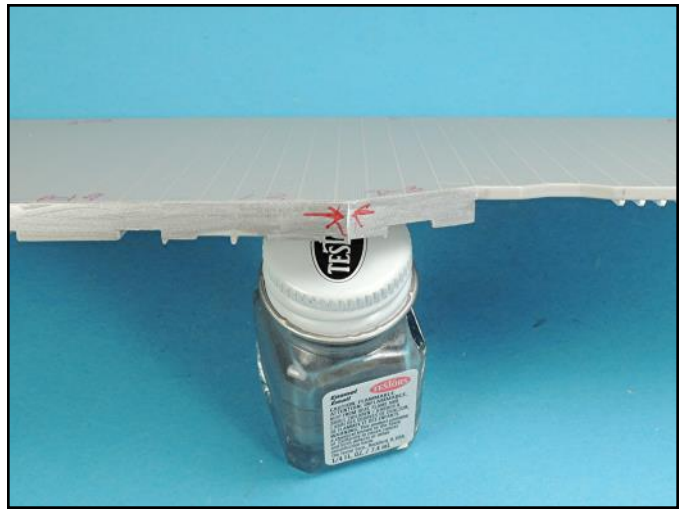
This edge was slightly distorted by sanding and it would not have been noticed except for the silver paint highlighting this problem.
