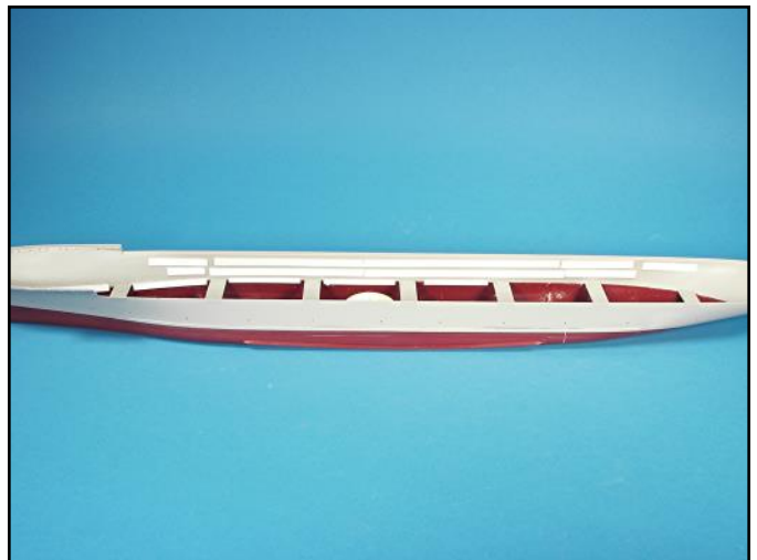
The hull is now ready for the next step - assembling the hanger deck. Laminating plastic strips to the inside areas of the hull stiffened the assembly, making it easier to work on the seams and prevented any cracking along the seam lines.
