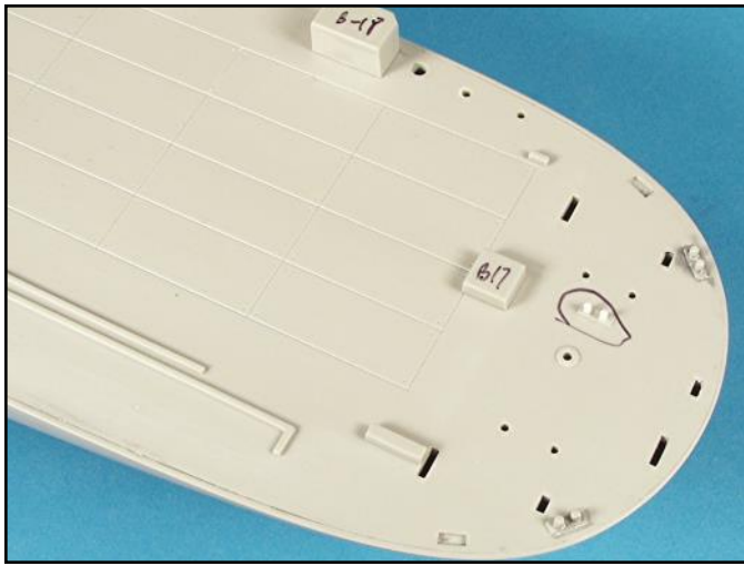
The deck bitts on the aft deck were broken off so they were replaced with plastic rod.
