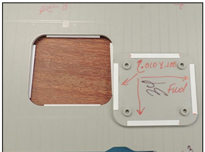
The flight deck elevators did not sit flush with the surrounding flight deck so shims were added to level both elevators.
