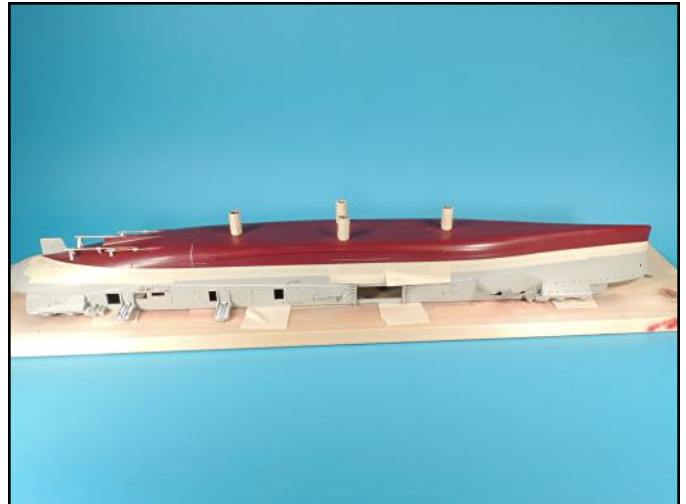
Long sections of masking tape with clean cut edges were applied along the demarcation line between the red hull color and the gray hull color.
