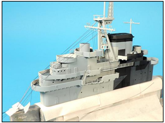
The island superstructure rigging was completed after the railings were attached and before the sub-assembly was glued to the flight deck.
