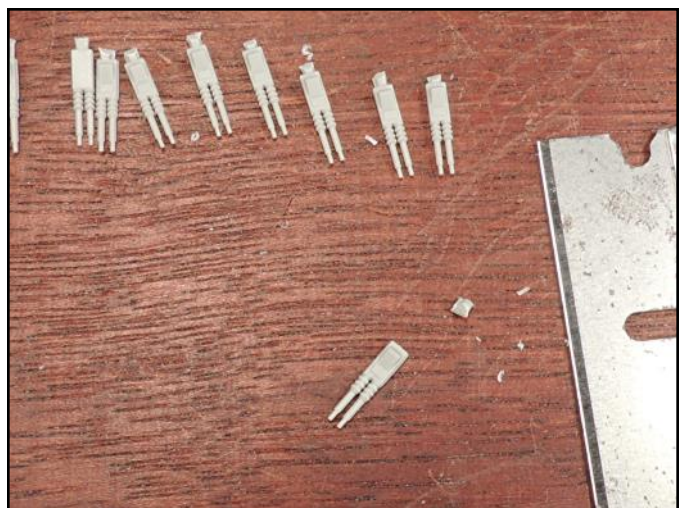
The tree attachment points on the 40mm guns were removed using a single edge razor blade. The single edge razor provided better positioning control to slice through the excess plastic.
