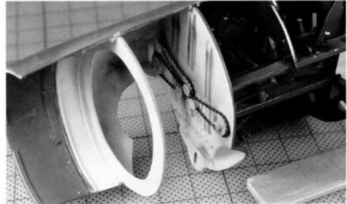
Fig. 4-72. Here the firewall has been installed and painted and the chain has been added. The chain really enhances the interior area of the landing gear bay, besides providing a high level of accuracy.
