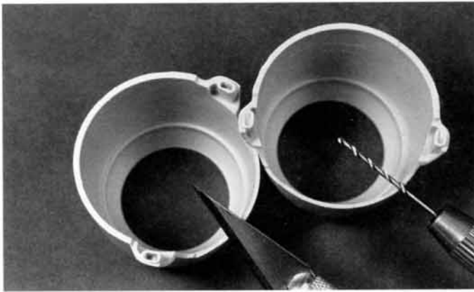
Fig. 4-37. Sometimes just deepening the exhaust ports can greatly enhance their appearance. These 1/48 scale A-20G Havoc exhaust ports will look a lot better once the inside areas are painted black and the cowlings are installed.
