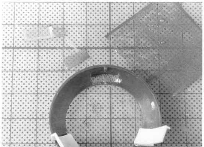
Fig. 4-24. Cut the screening to shape, insert it into the opening for the backside of the part, and glue it into place with a small amount of super glue.
