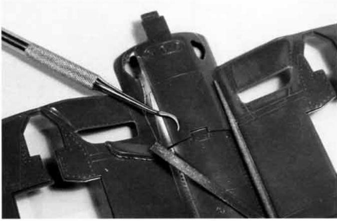
Fig. 4-31. The molded-on air outlets for this 1/32 scale F4U Corsair were removed with Bare Metal Foil's plastic scriber. The openings were then shaped with micro files.
