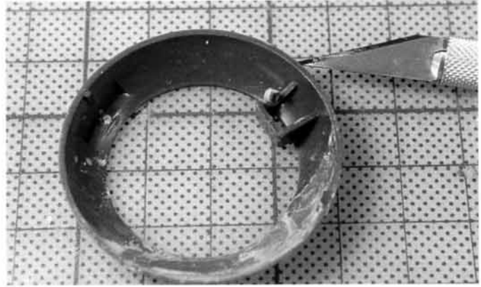
Fig. 4-26. To improve the appearance of large air intakes, such as the ones found on Revell's 1/32 scale F4F Wildcat aircraft, remove the molded-on air intakes. Such large molded-on detail can be removed by slowly peeling away the plastic with a no. 11 X-acto knife and then sanding the surface flat.
