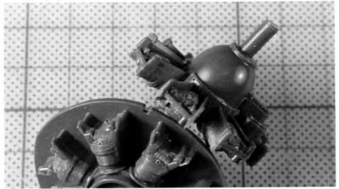
Fig. 4-8. In order to add wiring details to this engine, corresponding holes were drilled into the engine cylinders as well as around the rim of the engine case.
