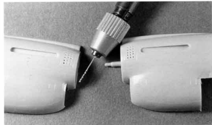
Fig. 4-30. The appearance of the engine breather holes on this 1/72 scale P-40 were greatly enhanced by drilling out the individual holes. This is yet another example of how a simple modification can greatly enhance the realistic appearance of any scale model.
