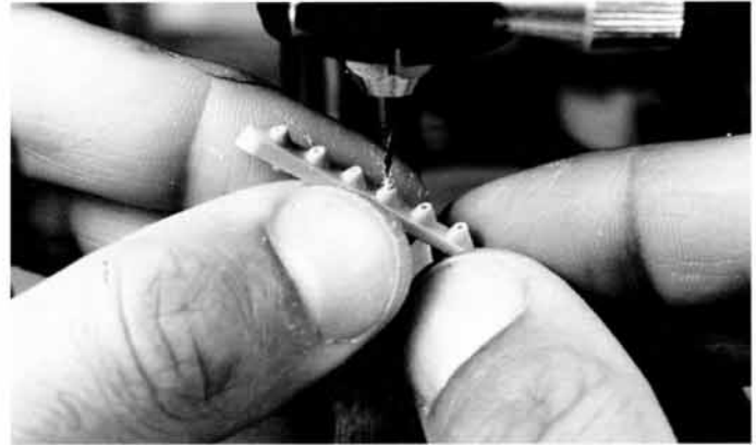
Fig. 4-34. Drilling out the exhaust ports is another simple enhancement that you can make. These exhaust ports are being drilled out using a Dremel drill press, although they could have just as easily been drilled out by hand.
