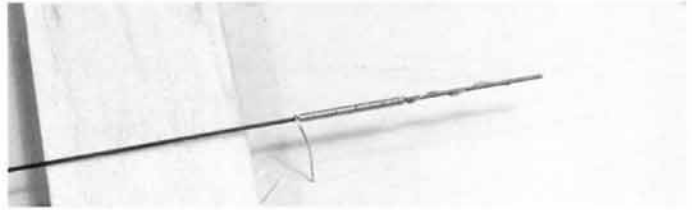
Fig. 4-44. Many different types of landing gear have large springs as part of the gear mechanisms, and these are easy to duplicate with soft brass beading wire wrapped around a stiff length of wire.
