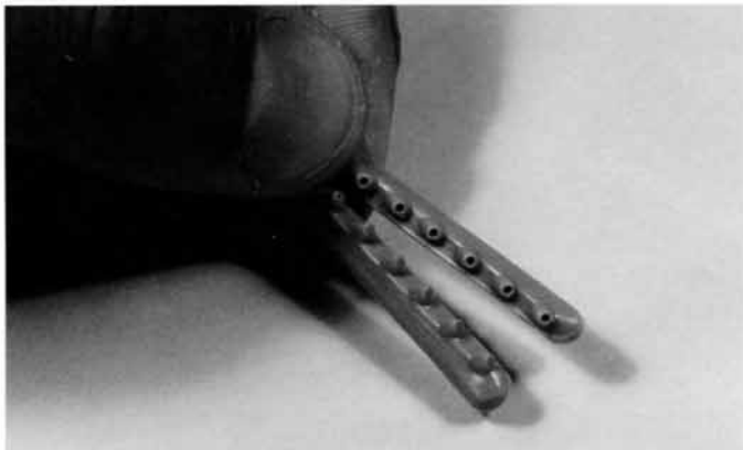
Fig. 4-35. Hollowing out engine exhaust ports on kit-supplied parts makes a big difference in their overall appearance.
