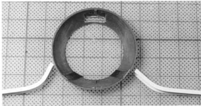
Fig. 4-27. To make new air intakes for this F4F, Evergreen channel stock was used. The plastic was softened by placing it against a 100-watt light bulb and then pushing against the interior cone shape of the cowling to shape it. The edges of the labeling tape acted as a locating lip for these parts as they were being form-fit into place.
