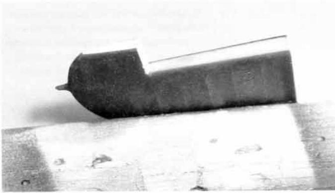
Fig. 5-18. Another good example of using resin to fill a control surface. Resin also adds a great amount of strength to these small parts by completely filling the cavity.
