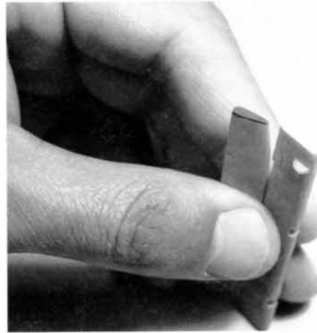
Fig. 5-22. Plastic was added to the edges of these control surfaces so that they would fit snugly into their openings. Don't forget to check for these small details.
