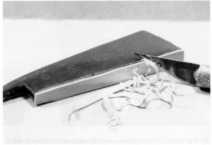
Fig. 5-13. Here the elevator opening has been sealed on this wing surface and the excess plastic has been slowly peeled off.
