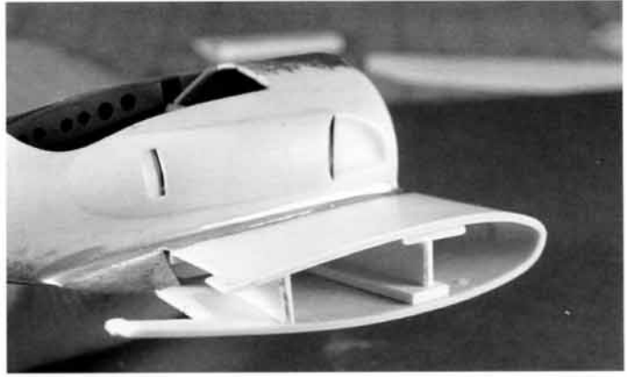
Fig. 5-7. Removing both the ailerons and flaps on wings can make them very fragile. I recommend that you add scraps of plastic to the inside area of the wing wherever possible to reinforce it.
