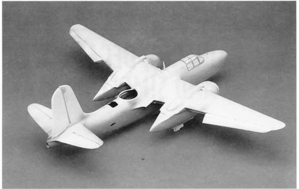
Fig. 5-37. With control surfaces attached and clear parts masked, this A-20G is ready for painting.
