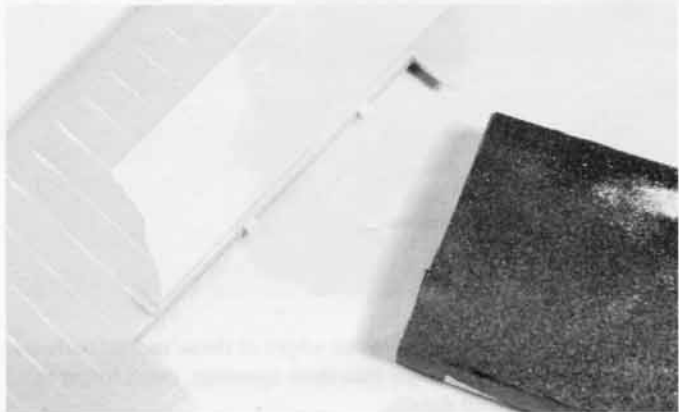
Fig. 5-24. The first step in adding hinges is to pick a strip stock size close to the hinge size that you want, install the hinges in the control surface, and tape it into place. Next apply a tiny amount of super glue to the back side of each hinge so that it is attached to the wing.
