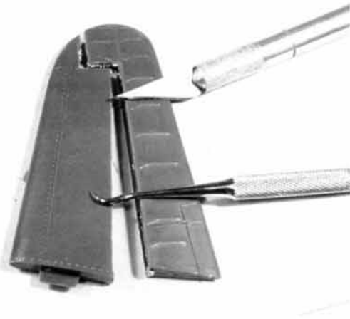
Fig. 5-1. There are several different ways to remove control surfaces; the method you use depends on the situation. In most cases using Bare Metal Foil's plastic scribe to cut most of the way through the plastic and then using a sharp no. 11 X-acto blade to cut the rest of the way through works very well.
