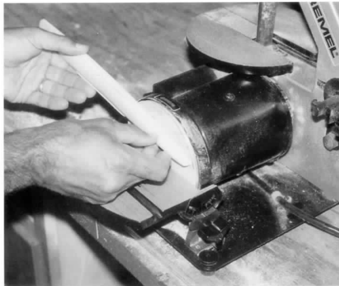
The first step in assembling a resin ship hull is to remove the pour plug if there is one. The easiest way to do this is with a disk sander. Be careful that you don't oversand, and check your work frequently.
