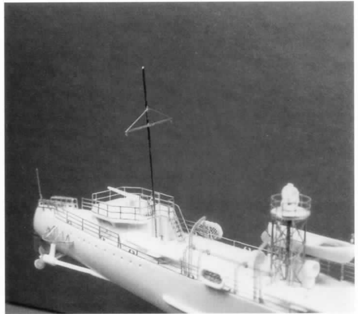
Set up the rear mast on the same model with a thin-diameter length of brass wire and a photoetched yardarm. With small-diameter wire there is no need to contour its length.
