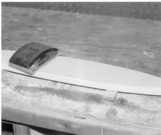
Some resin manufacturers like Classic Warships don't have resin pour plugs on their ship hulls, but you still have to flatten the gluing surface. The easiest way to do this on large models is with a hand sander.
