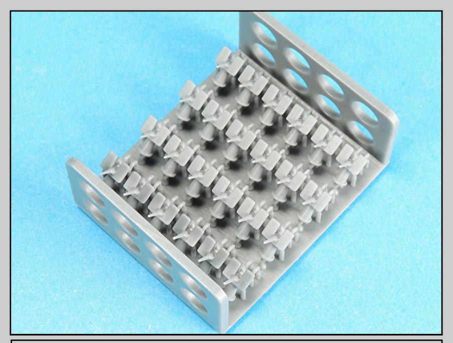
The gun barrels and shields are beautifully printed with no residue around the tips or the edges.
