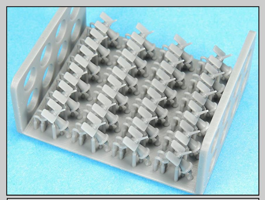
Here again note how tiny the diameters are on the tree attachment points on each gun are. This makes it very easy to remove any remaining stubs with the tip of a number 11 X-Acto blade.
