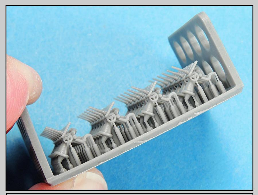
The adjusting wheels are spoked and the gun bases are very clean with no resin residue. Note how the tree connectors between the part and the base get smaller in diameter.
