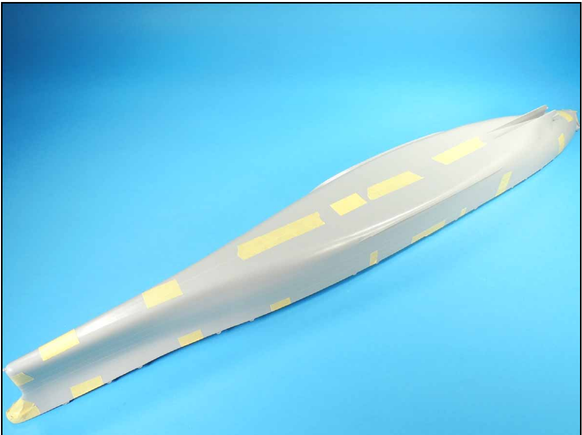
The seam line on the hull is approximately 32.5 inches long.
