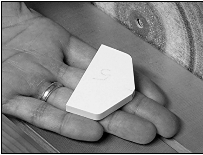
The block is now shaped to the dimensions of the superstructure part. To smooth the surfaces I run them across waterproof sandpaper from 400 to 600 grit and I wet sand the plastic.
