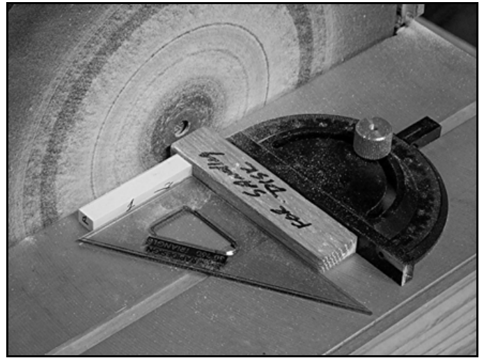
Narrow sections can be shaped with the help of blocks of wood and drafting triangles.
