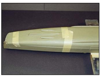
Here is the opposite side of the hull and while the edges are almost lined up there is also a shrinkage problem with the length of the part as well as its width.
