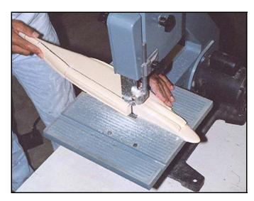
The longer cuts take a steady hand. Be sure that the band saw base is level and at 90 degrees to the saw blade. The blade will cut through resin like a hot knife through butter, so be careful when cutting.
