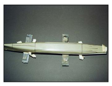
I outline where cuts in the hull need to be made to allow the edges of the lower hull to mate up with the edges of the upper hull, using an indelible marker.
