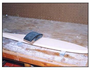
The first step in attaching the upper and lower hulls is to remove any excess casting material. If you do not wet sand be sure to wear a dust mask as the resin particles can irritate your lungs.
