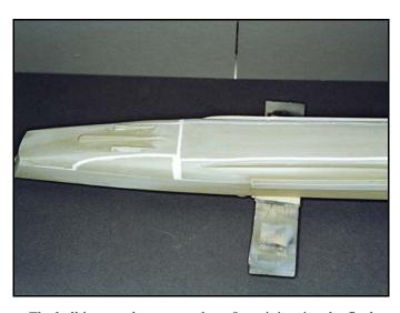
The hull is now almost complete. Once it is primed a final check will be made to fill any remaining imperfections and voids.
