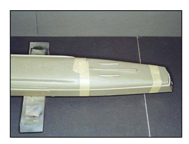
This is a good example of the shrinkage that can occur on resin hull halves. There is no way these parts can be mated together.
