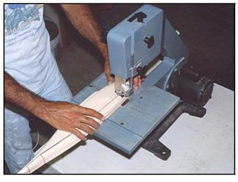
Here is where steel nerves are needed. I cut the lower hull up using a band saw! I make the short cuts first. Be sure to wear a dust mask as the resin particles go all over the place!
