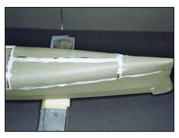
To help fill any remaining gaps between the upper and lower hull I added tiny amounts of resin. One of the great qualities of resin is that new resin sticks to old resin which makes it a great filler!
