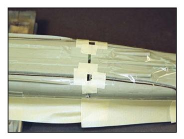
Here is a close up of the packaging tape. You need to make sure that the tape is attached to the edges of the openings so that resin will not seep out onto the surface of the hull. Also note the openings locations for pouring resin.
