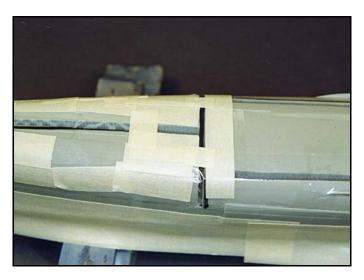
I use masking tape to outline the openings and to protect the surrounding areas from over pours of the liquid resin. Also, be sure to put the packaging tape along the seam line between the upper and lower hull.
