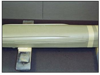
Here you can see how one side almost lines up while the other side close to the bow had both shrinkage and a wrap. Most modelers would decide to make a waterline model but there is another way, surgery!
