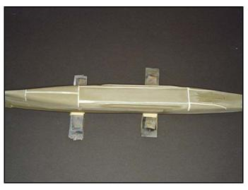
An initial wet sanding smoothed out the resin pours and helped contour it into the shape of the hull.
