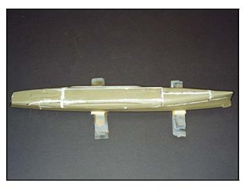
The resin was carefully mixed in small batches and poured into the openings. It looks a bit messy, but all the openings and tiny voids have been filled. The resin even seeped into the areas along the seam line between the hulls halves.
