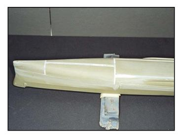
The completed hull looks a lot better! Finer grits of sandpaper are being used to smooth out the resin and contour it into the hull. Always remember to wet sand resin.
