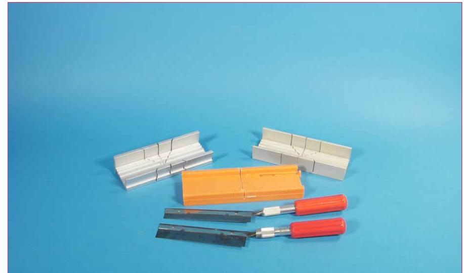
Miter boxes and razor saws are necessary for cutting plastic stock. These miter boxes are specifically designed for razor saws. Razor saws also come in various cutting grades.
