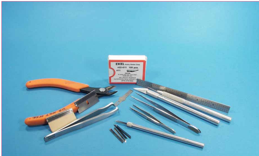
Here are the basic hand tools for snipping, cutting, trimming and scraping. The small diameter X-Acto handle and associated blades is a stencil knife. I always keep a good supply number 11 X-Acto blades on hand as well as a box of single edge razor blades and other specialty blades. The stainless steel ruler, can be found in sewing supply stores. The Tweezers and the needle tool all have a thousand and one uses in scale modeling.
